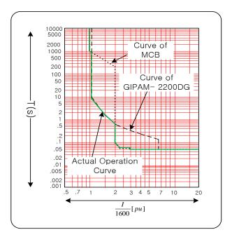
Figure 3. Present coordination curve of OCR for generator.
