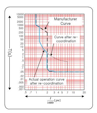
Figure 5. Re-coordination curve of the OCR for generator.
