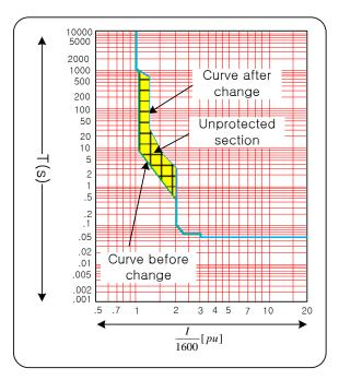
Figure 6. Actual OCR curves after and before re-coordination.
