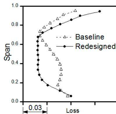
**Figure 18.** Loss profiles of the baseline and redesigned stator 5 (near the stall points).
