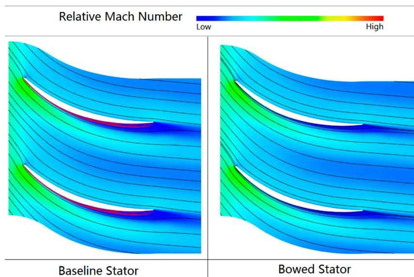
**Figure 14.** Relative Mach number contours and streamlines at the 35% span of stator 5 (near the stall points).
