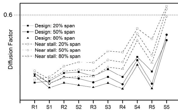
Figure 8. Streamwise diffusion factor distributions of each row.
