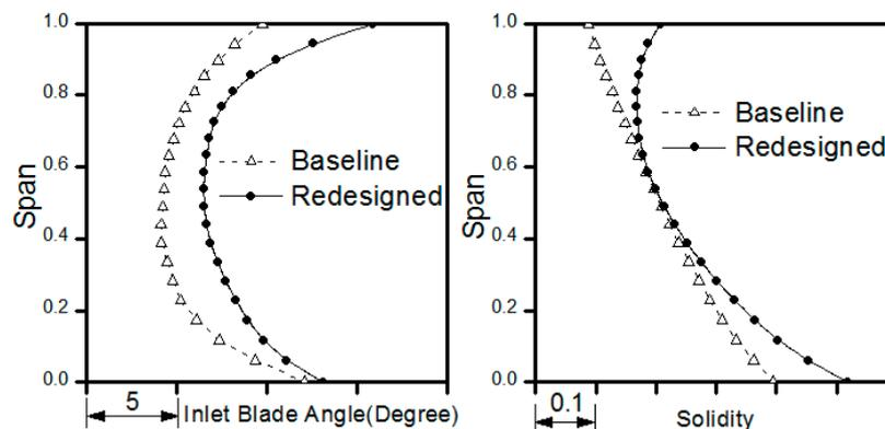
Figure 16. Inlet blade angle and solidity profiles of the baseline and redesigned stator 5.
