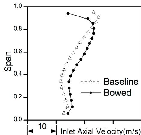
**Figure 12.** Spanwise distributions of the inlet axial velocity (near the stall points).
