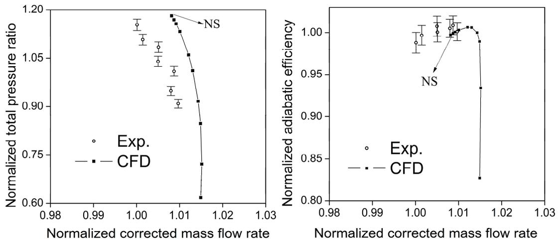
Figure 4. Measured and predicted overall performance. NS: Near Stall.
