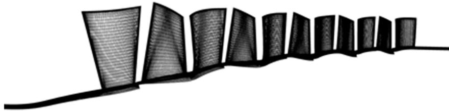
**Figure 3.** Mesh for the CFD computations.
