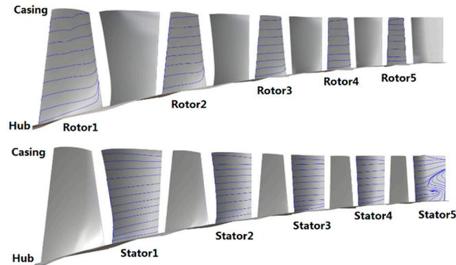
Figure 7. Limiting streamlines on the suction side of each blade at the near stall point.
