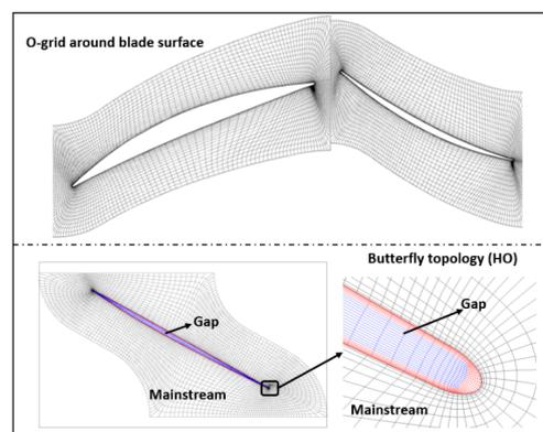
Figure 2. Typical mesh topology.
