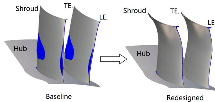
**Figure 20.** Iso-surface of the axial velocity ( $-1$  m/s) for the baseline and redesigned stator 5 (near the stall points).
