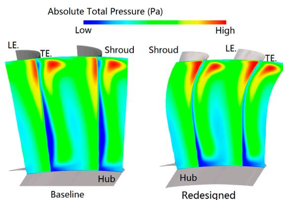
**Figure 19.** Total pressure contours downstream of the baseline and redesigned stator 5 (near the stall points).
