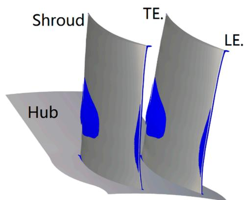
**Figure 10.** Iso-surface of the axial velocity ( $-1$  m/s) for stator 5 of the baseline (near the stall points). TE.: trailing edge; LE.: leading edge.
