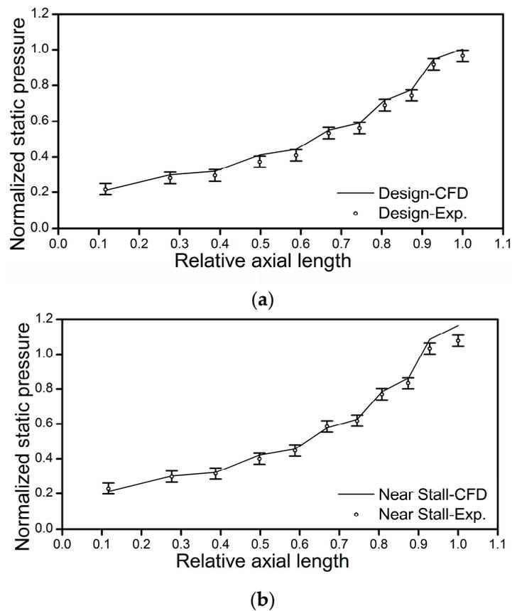
Figure 5. Measured and predicted casing static pressure. (a) Design point; (b) Near stall point. Exp.: Experiment.
