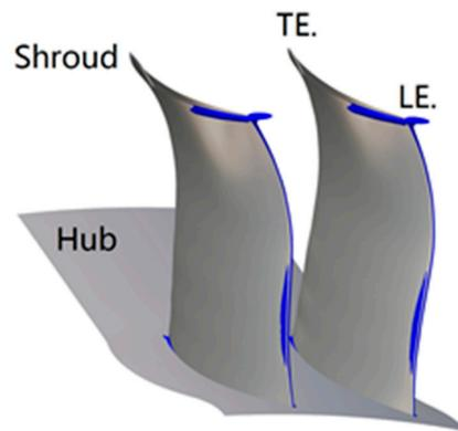
**Figure 13.** Iso-surface of the axial velocity ( $-1$  m/s) for the bowed stator 5 (near the stall points).
