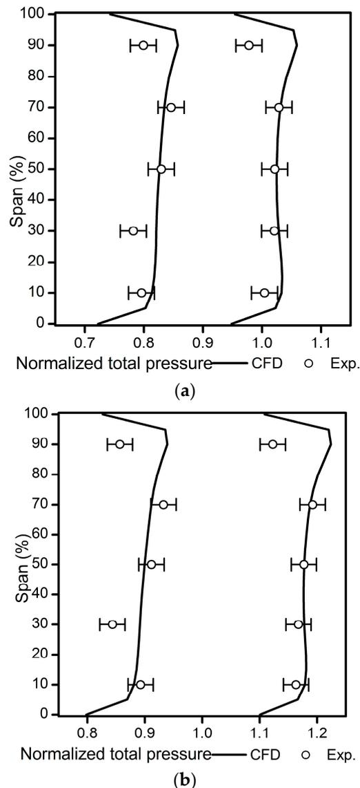
**Figure 6.** Measured and predicted total pressure profiles at the leading edges of stator 4 and stator 5. (a) Design point of stator 4 and stator 5; (b) Near stall point of stator 4 and stator 5.
