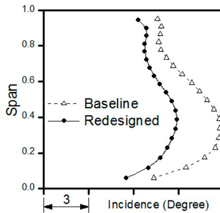
**Figure 17.** Spanwise distributions of the incidence for the baseline and redesigned stator 5 (near the stall points).
