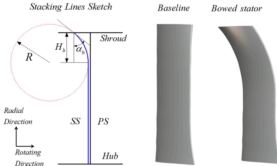
**Figure 11.** Stacking lines sketch and blade shapes of stator 5. SS: suction side; PS: pressure side.
