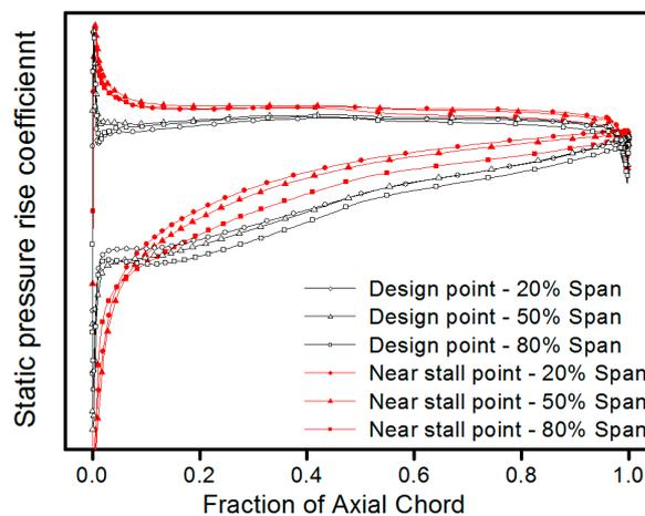
Figure 9. Surface static pressure rise coefficient distributions at the 20%, 50% and 80% spans of stator 5.
