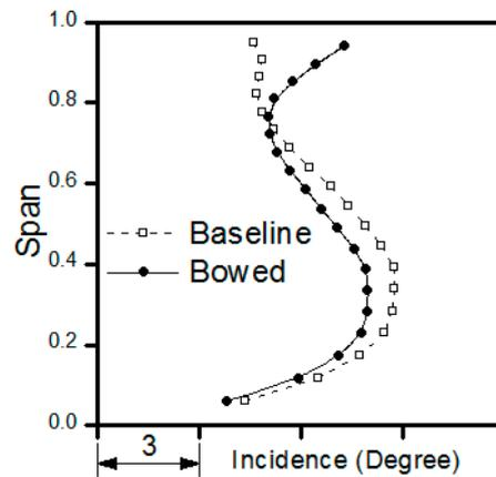
Figure 15. Spanwise distributions of the incidence at the design point.
