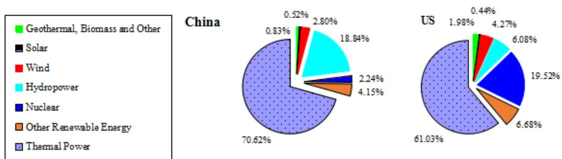
Figure 7. Comparison of renewable energy consumption in 2014 between China and the US.
