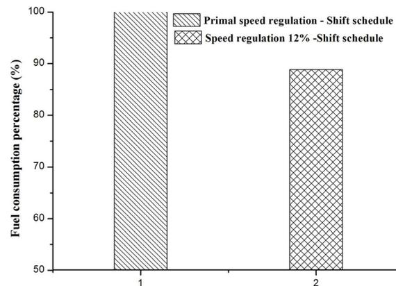
**Figure 15.** Fuel consumption percentage of real vehicle confirmatory experiment in the smooth driving cycle.
