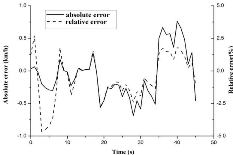
Figure 11. Error between the simulation velocity and the real velocity.
