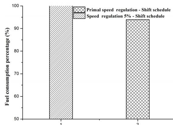
**Figure 16.** Fuel consumption percentage of real vehicle confirmatory experiment in the complex driving cycle.
