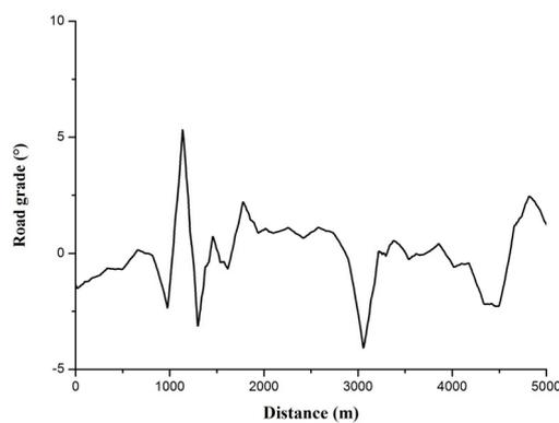
Figure 8. Complex driving cycle (road grade-distance).
