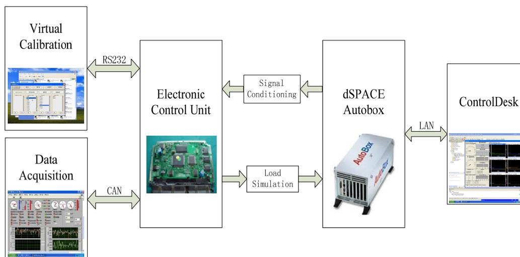
**Figure 1.** Virtual calibration platform.
