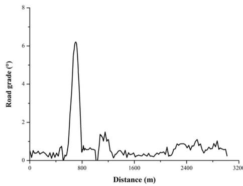
Figure 6. Smooth driving cycle (road grade-distance).
