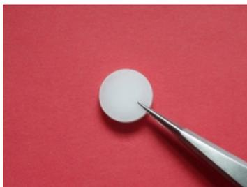
**Figure S2.** Photograph of pressed shaped  $\text{Al}(\text{NH}_2\text{BH}_3)_3 \cdot 3\text{NH}_3$  powder after exposure to dry air for 3 days.
