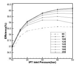
Figure 11. Effect of IPT inlet pressure on efficiency given different HPT inlet pressures.
