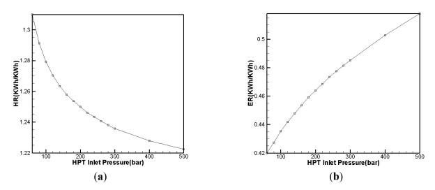
Figure 8. Effects of HPT inlet pressure on (a) heat rate (HR); (b) electric power consumption rate (ER).
