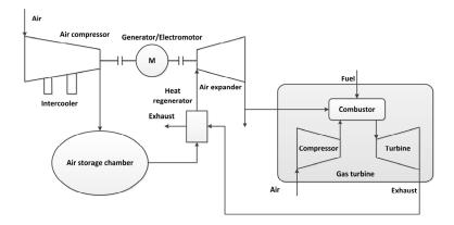
Figure 3. Schematic of the second-generation CAES power system.
