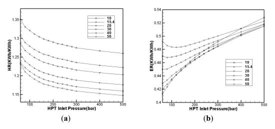
Figure 10. Effects of HPT inlet pressure on (a) HR and (b) ER under different IPT inlet pressures.
