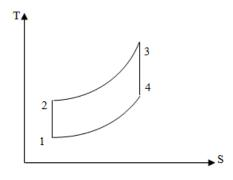
Figure 4. T-S (Temperature-Entropy) chart of the Brayton cycle.
