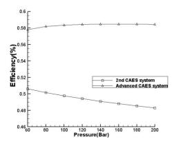
Figure 14. Effect of changes inair storage chamber pressure on efficiency.
