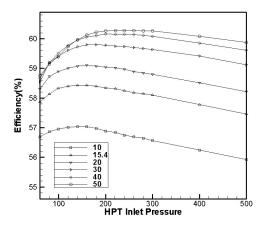
**Figure 9.** Effects of HPT inlet pressure on efficiency under different intermediate pressure turbine (IPT) inlet pressures.
