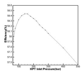
Figure 7. Effects of high-pressure turbine (HPT) inlet pressure on efficiency.
