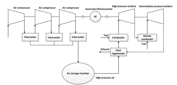
Figure 6. Schematic of the improved CAES system.
