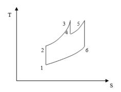
Figure 5. T-S chart of the reheat Brayton cycle.
