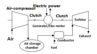
Figure 2. Compressed air energy storage (CAES) power generation system.
