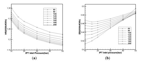
Figure 12. Effect of IPT inlet pressure on (a) HR and (b) ER given different HPT inlet pressures.
