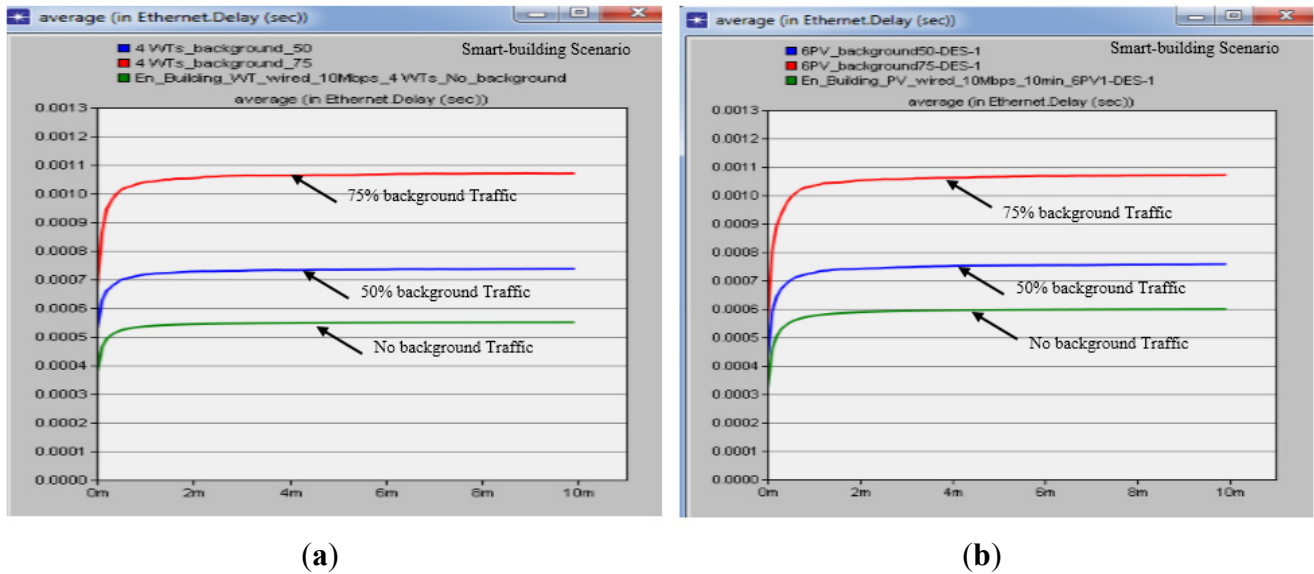
Figure 14. (a) Average ETE delay of Ethernet-based architecture for four WT; (b) Average ETE delay of Ethernet-based architecture for four PVs.
