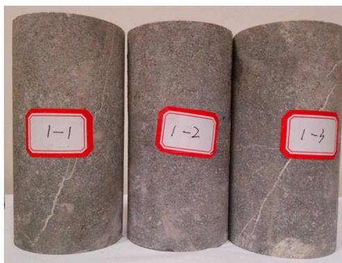
Figure 6. Specimens in acoustic emission test.
