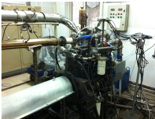
Figure 10. Test bench of YC4E170-31 diesel engine.
