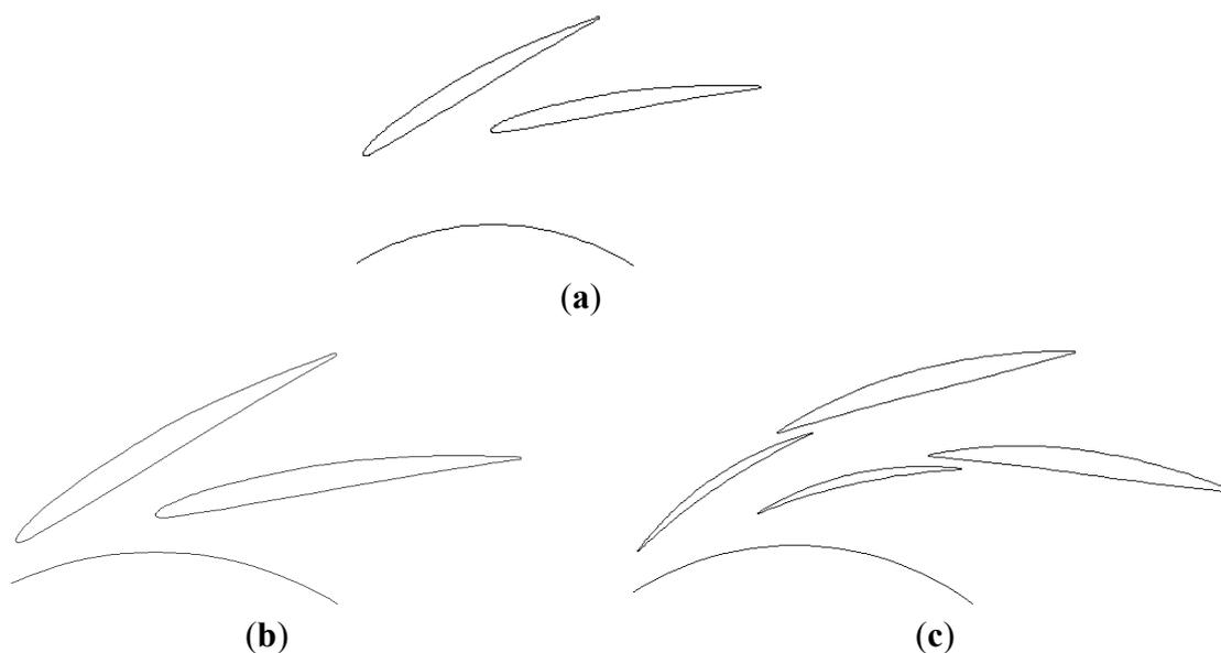
**Figure 7.** Geometric structure of the vaned diffuser: (a) Original design; (b) Optimization design 1; (c) Optimization design 2.
