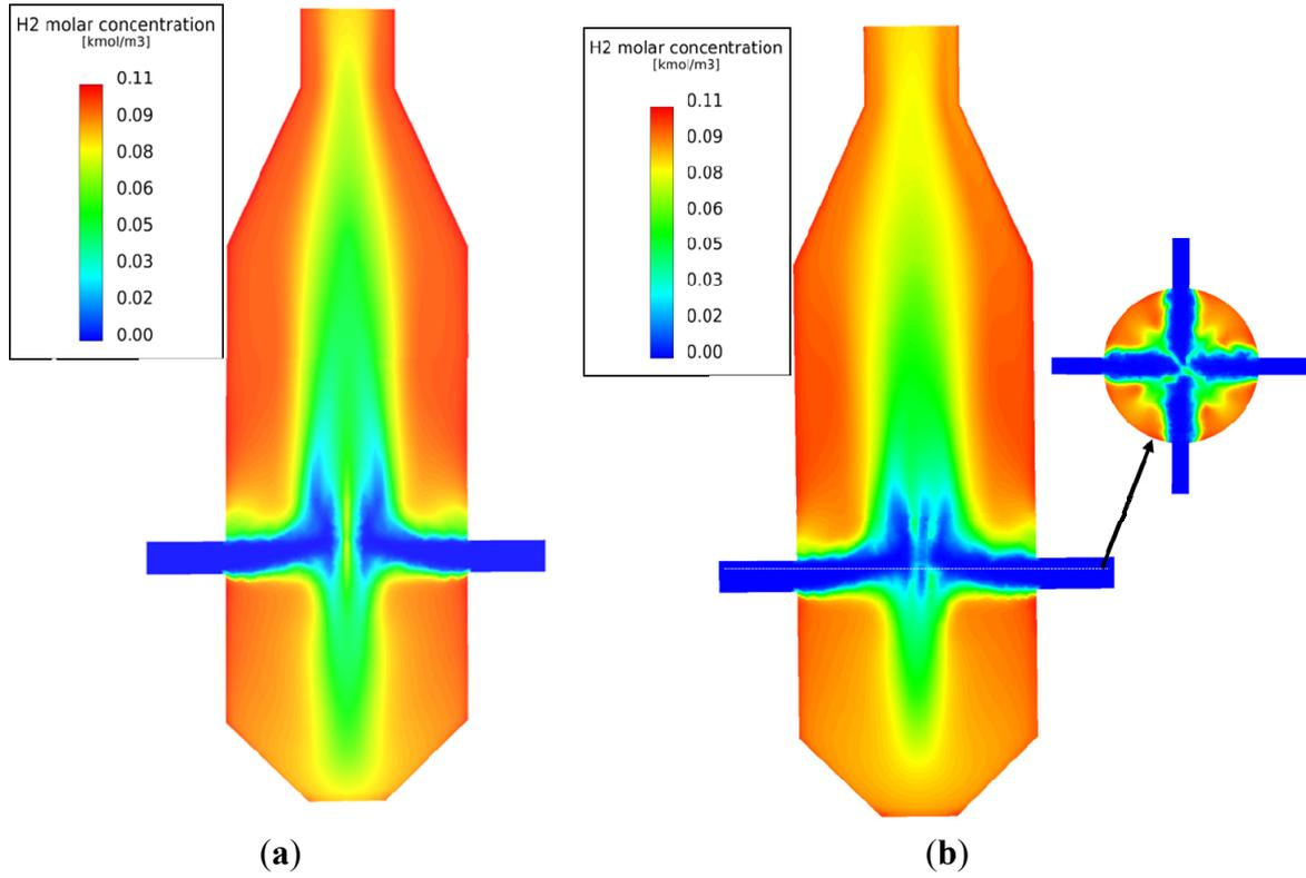
**Figure S8.** Distribution of H<sub>2</sub> molar concentration for 1/4 periodic and whole geometries. (a) 1/4 periodic geometry; (b) Whole geometry.
