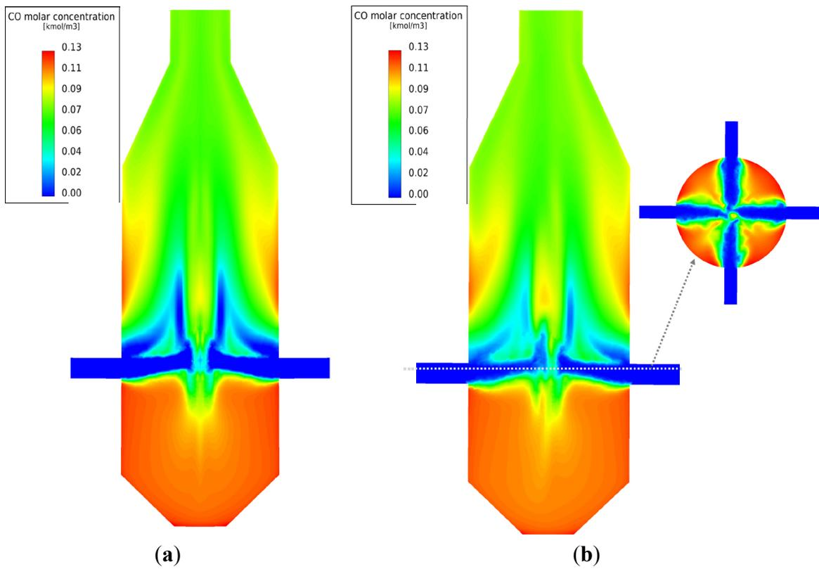
**Figure S6.** Distribution of CO molar concentration for 1/4 periodic and whole geometries. (a) 1/4 periodic geometry; (b) Whole geometry.
