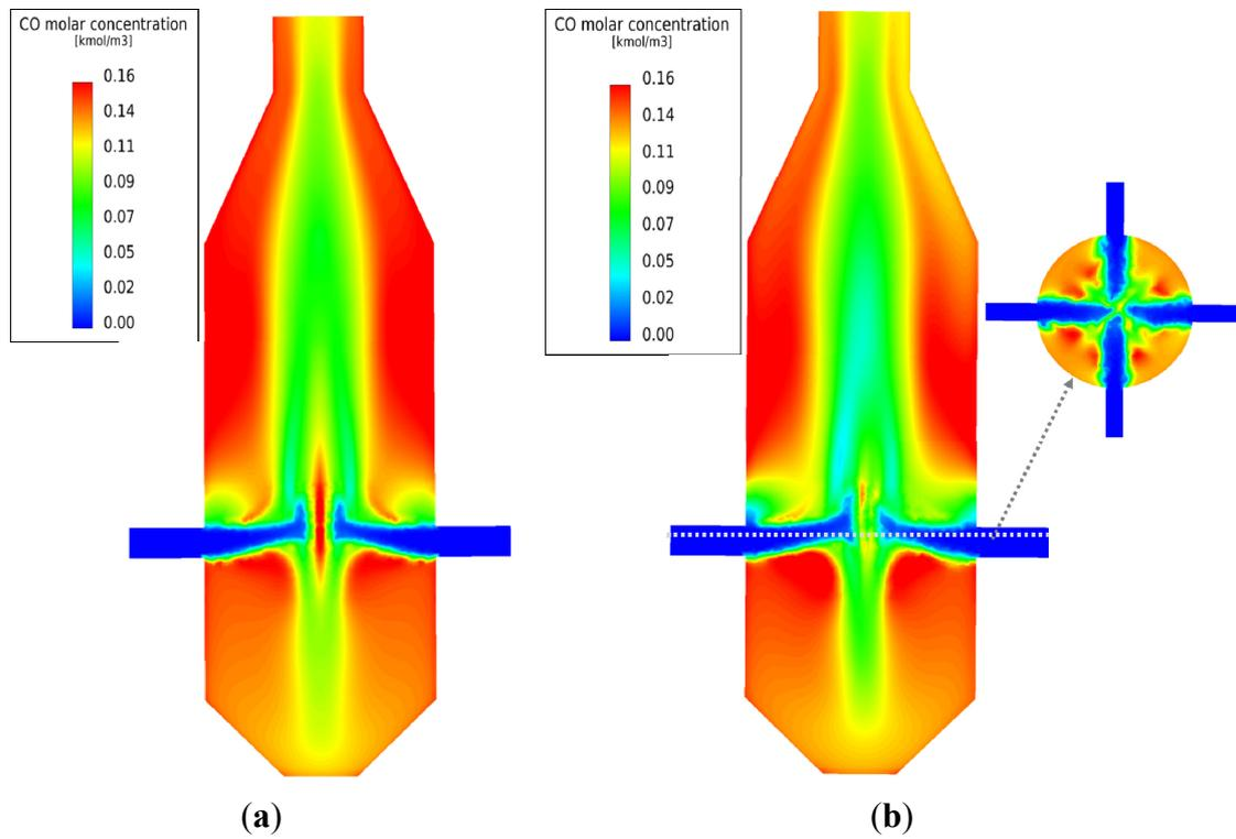
**Figure S9.** Distribution of CO molar concentration for 1/4 periodic and whole geometries. (a) 1/4 periodic geometry; (b) Whole geometry.
