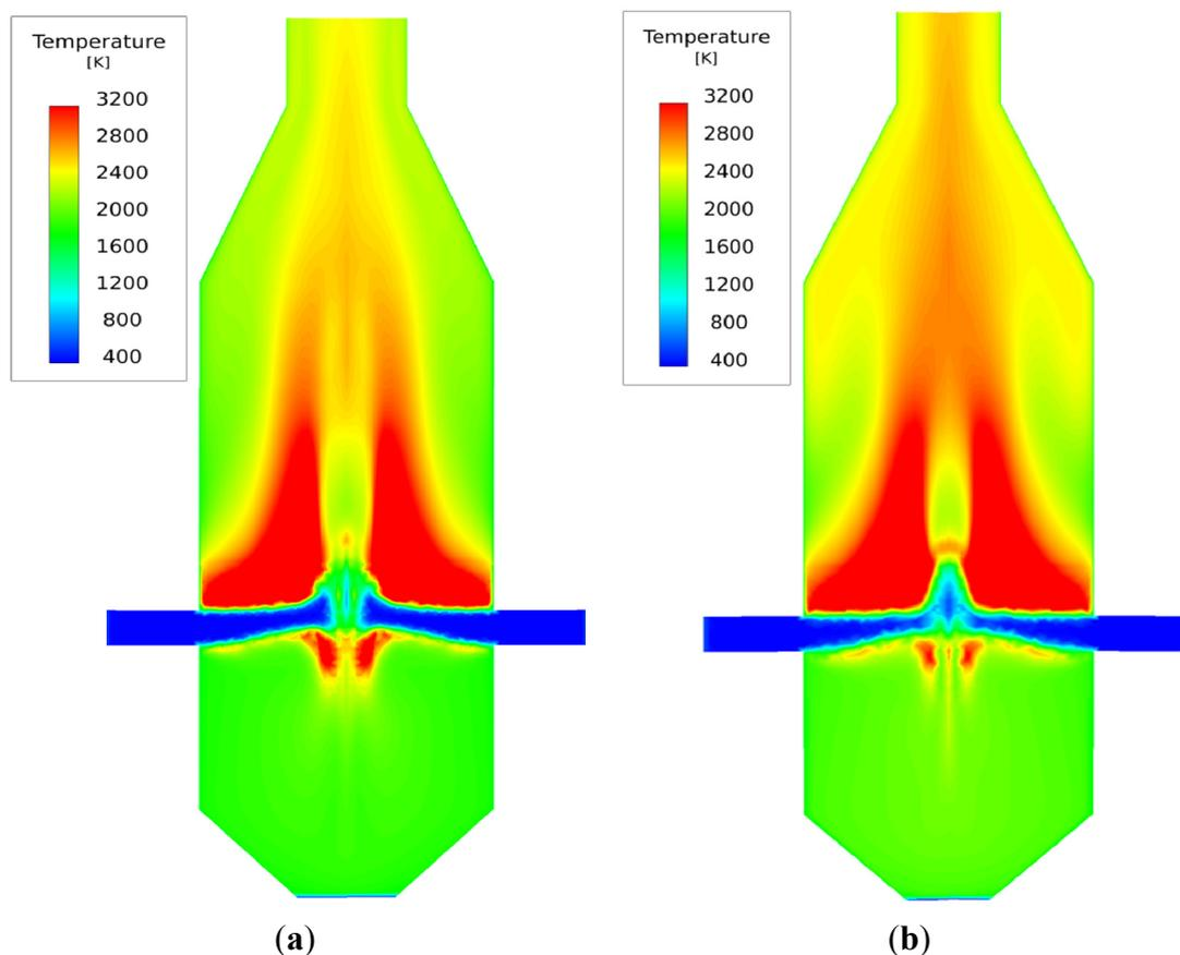
**Figure S1.** Distribution of temperature for DO and P-1 radiation model. (a) DO radiation model; (b) P-1 radiation model.
