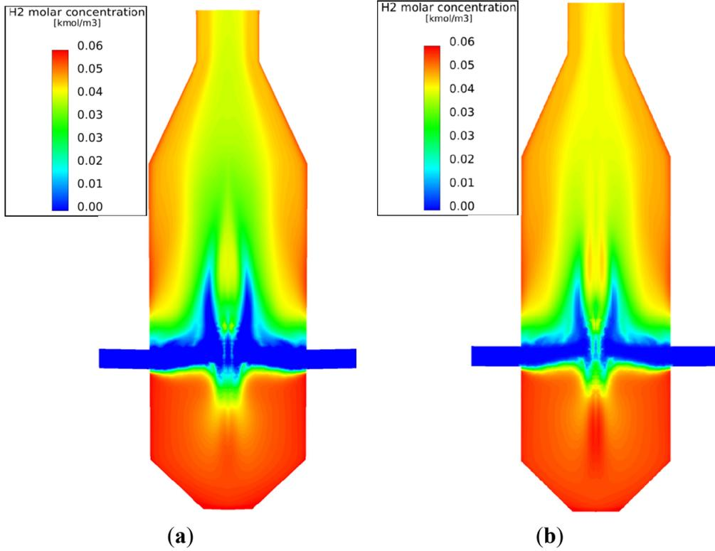
**Figure S2.** Distribution of H<sub>2</sub> molar concentrations for DO and P-1 radiation model. (a) DO radiation model; (b) P-1 radiation model.
