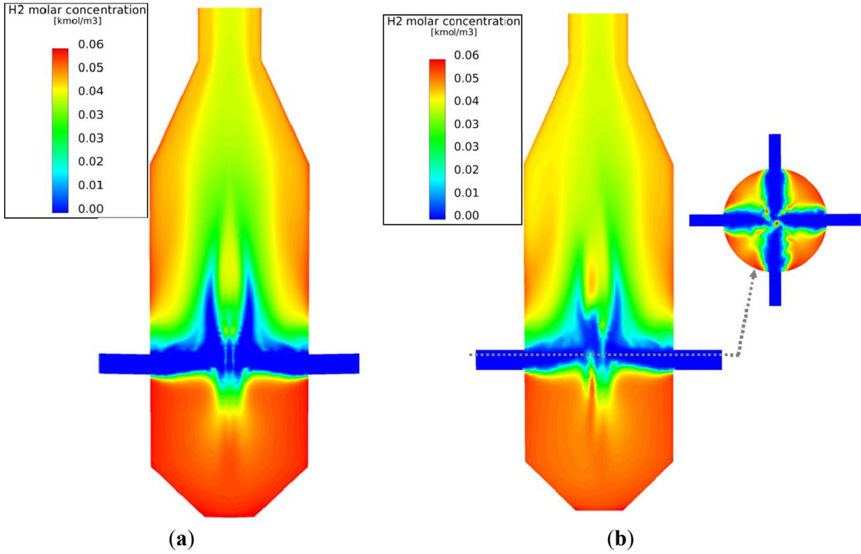
**Figure S5.** Distribution of H<sub>2</sub> molar concentration for 1/4 periodic and whole geometries. (a) 1/4 periodic geometry; (b) Whole geometry.
