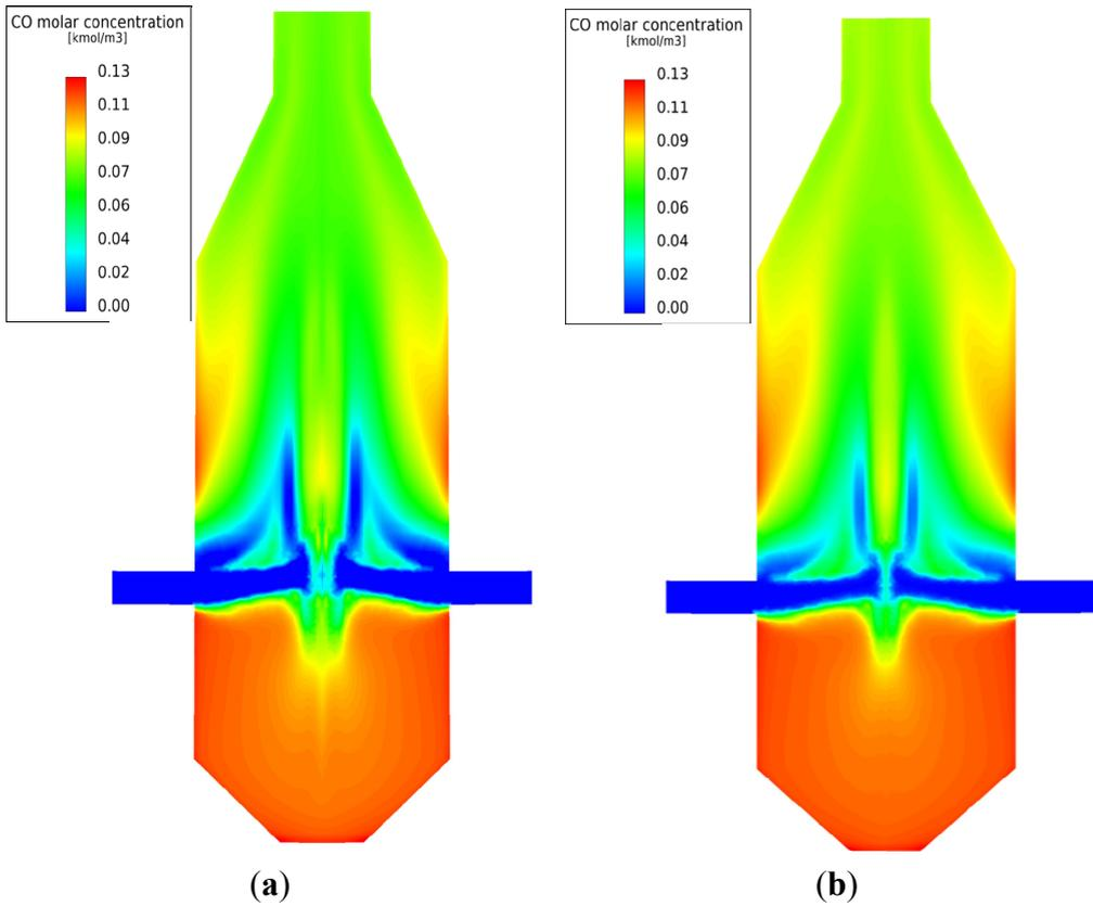
**Figure S3.** Distribution of CO molar concentrations for DO and P-1 radiation model. (a) DO radiation model; (b) P-1 radiation model.
