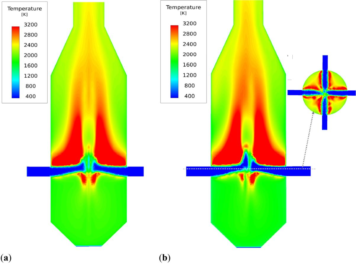
**Figure S4.** Distribution of temperature for 1/4 periodic and whole geometries. (a) 1/4 periodic geometry; (b) Whole geometry.
