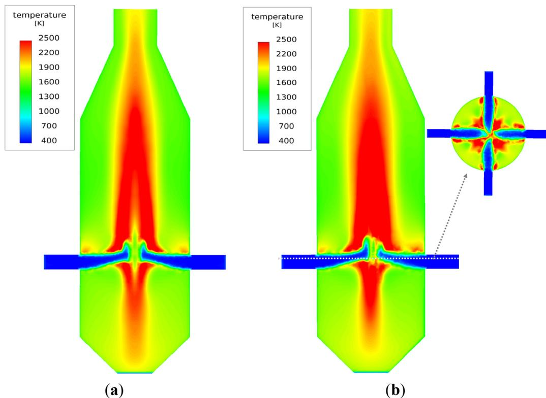
**Figure S7.** Distribution of temperature for 1/4 periodic and whole geometries. (a) 1/4 periodic geometry; (b) Whole geometry.
