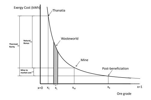
**Figure 3.** Thermodynamic rarity represents the exergy cost (kWh) needed for producing a given mineral commodity from bare rock to market, *i.e.*, from Thanatia to the mine and then to post beneficiation.
