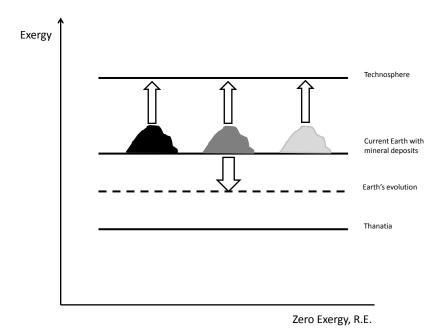
**Figure 1.** Graphical representation of the exergy associated with the minerals in the technosphere, the mineral deposits and Thanatia with respect to the reference environment.
