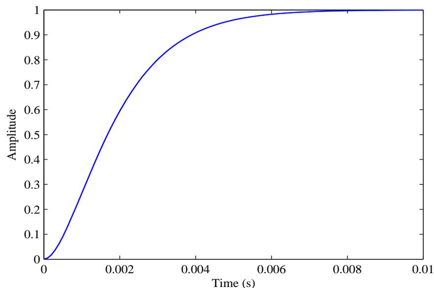
The controller,  $R_{v_{dc}}(s)$ , must be designed to obtain a time response that is much slower than the inner control loop response. Under this design constrain, the controller gains are calculated by ignoring the dynamics of the inner control loop. In this case study, the desired locations of the poles of the closed-loop
