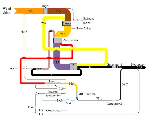
Exergy losses amount to 35.0 kW in total, with a split of 34.7 kW for the exhaust gases and 0.3 kW for the ash. The exergy losses associated with the discharged ash are negligible, while the ones with exhaust gases range between 4.5% and 6.5% of the total exergy input of the plant.
