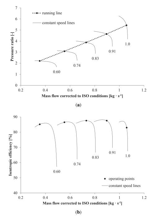
Figure 8(a) and 8(b) illustrates the maps and the corresponding running line of the radial turbine mechanically coupled to the centrifugal compressor. Given a reduction of the power output from 100%
