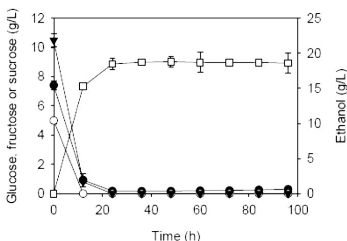
**Figure 2.** Time course of ethanol (□), glucose (●), fructose (○), and sucrose (▼) during the SSF process with 15% (w/v) carrot pomace as the feedstock. The initial carrot pomace charge was 10% (w/v) and an additional 5% (w/v) was added at 12 h.
