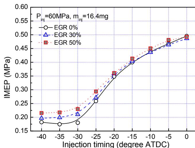
In addition, as the injection timing advanced, the differences in IMEP caused by the application of EGR increased. It can be concluded that longer ignition delays and prolonged combustion durations for EGR combustions improved the conversion of combustion heat into the effective work process.
