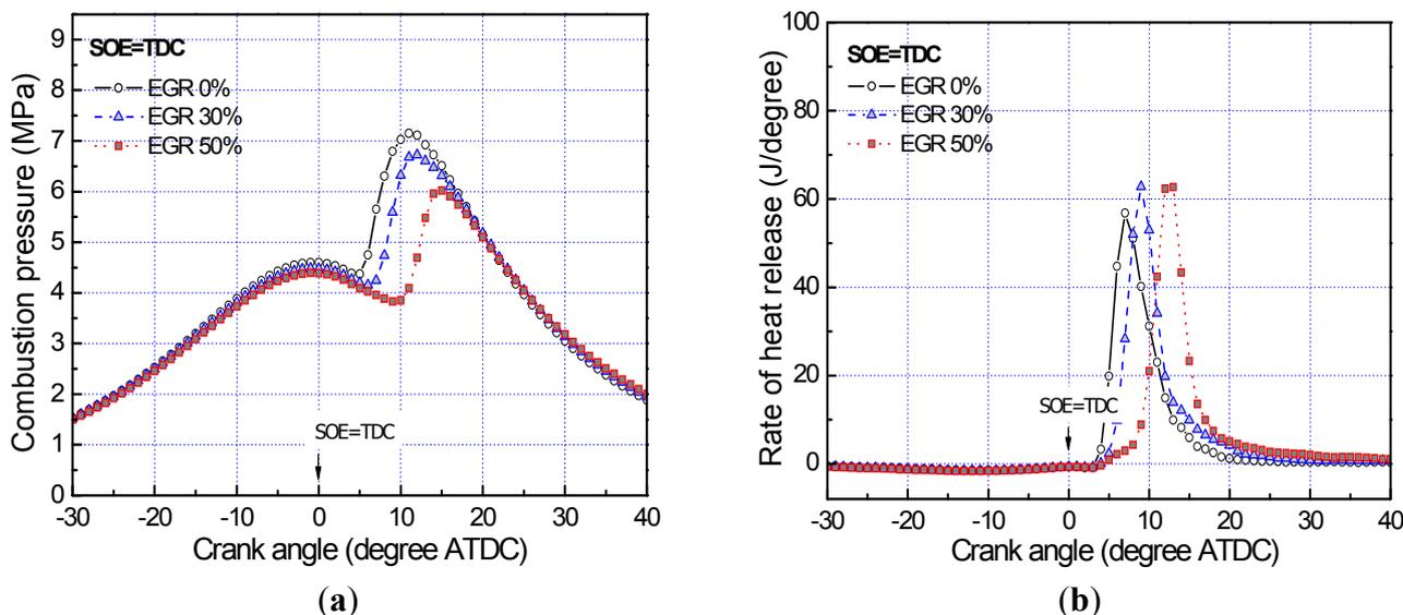
**Figure 3.** Effect of EGR rate on combustion performance characteristics with injection timing of BTDC 30°. (a) Combustion pressure; and (b) Rate of heat release (HRR).
