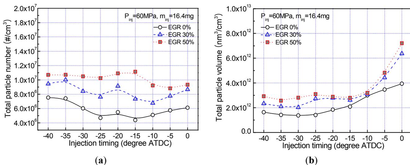
The simultaneous increase of particle number and volume may be due to concurrent processes of coagulation with homogeneous nucleation of metallic ash particles and heterogeneous nucleation of PAH and carbon soot on the metallic ash particle [18,19]. The engine operating conditions of EGR rate and injection timing can be optimized to minimize the particle emission characteristics of total particle number, particle volume and FSN results.
