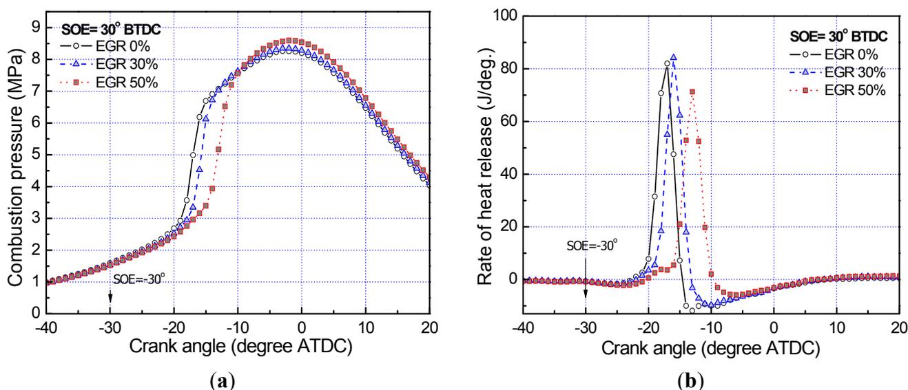
Figure 4 showed that the use of EGR slightly increased the IMEP because the heat of combustion was released between the end of compression stroke and the beginning of expansion stroke due to the prolonged ignition delay and combustion duration (recall Figures 2 and 3).
