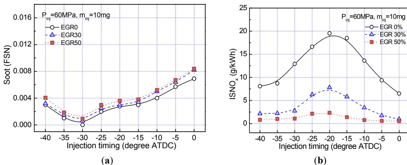
In general, both soot formation and soot oxidation mechanisms are a function of combustion temperature and net soot release is maximized when the two mechanisms equally compete with each other. A decrease in combustion temperature due to higher EGR rate resulted in a significant reduction of soot formation in the engine than soot oxidation in the cylinder because insufficient oxygen
