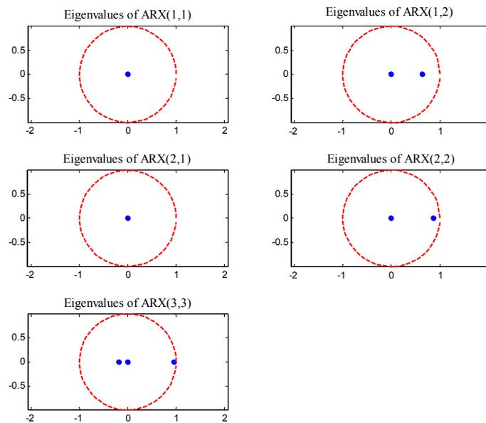
We conduct the stability analysis of the five proposed ARX models based on the stability Equations (15,16), and the roots distribution of these models are presented in Figures 14 and 15. The graphic results show clearly that the eigenvalues of the characteristic equations of the five models are all located inside the unit circle. Therefore, all five ARX models are stable.
