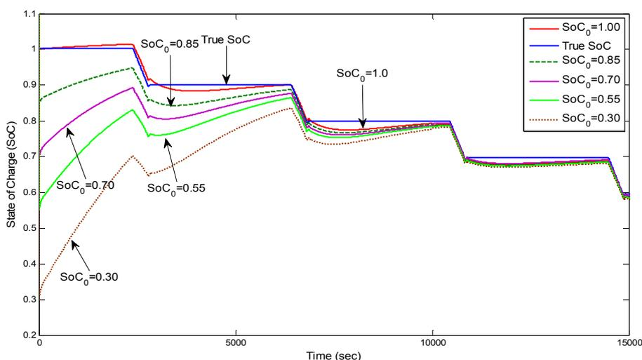
**Figure 23.** SOC curves for ARX(2,2) + EKF estimation with different initial SOC values ( $Q_{sk} = [1e-6], R_k = [1e-1]$ ) (full view).
