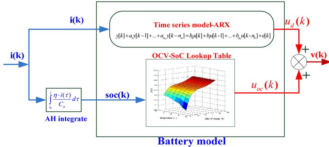
As seen in Figure 8, the battery model consists of two main parts: one is the open-circuit voltage (OCV), denoted as  $u_{oc}$ , which is modeled by a look-up table; another is the dynamic effect voltage, denoted as  $u_d$ , which is modeled by the ARX form. The explicit content of each part will be illustrated separately in the following subsections.
