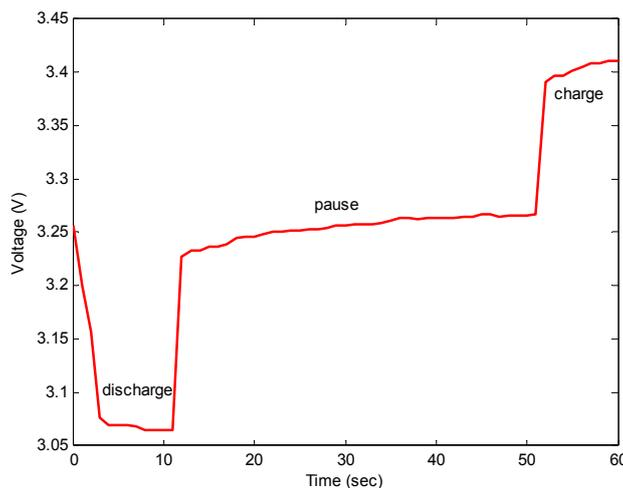
In order to identify the model parameters, hybrid pulse power characterization (HPPC) [12–14] tests were consecutively conducted with the lithium-ion battery module at each 10% SOC decrement across the range from 100% to 0%, while the temperature was maintained within  $25 \pm 0.5$  °C. One HPPC test profile at SOC = 50% is shown in Figure 5. Figure 6 displays the terminal voltage profile of
