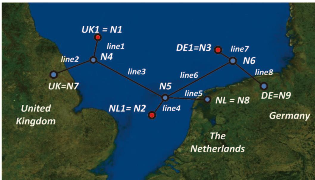
Each country has its own offshore wind farm (the red dots in Figure 1) named *UK1*, *NL1* and *DE1*. The black lines represent a pair of HVDC transmission cables and the intermediate nodes—*N4*, *N5* and *N6*—are cable T-joints. The wind farms size and location are derived by clustering the main offshore wind farms in the North Sea southern part; it includes wind farms in construction and planning phase.
