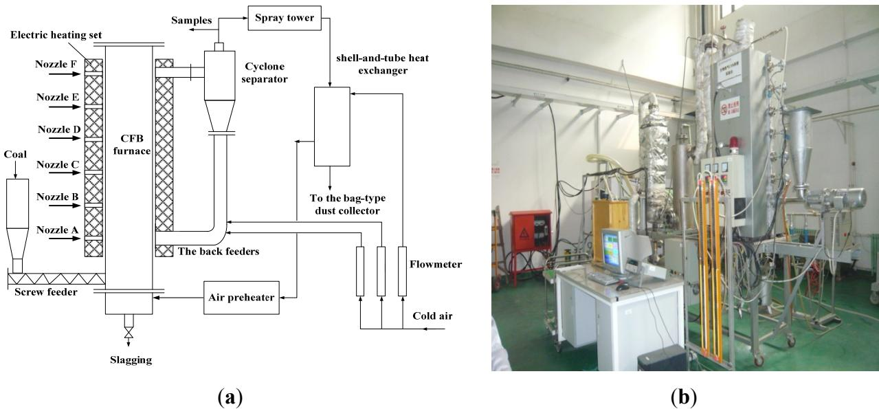
**Figure 3.** Fixed bed gaisifer subsystem for biomass gasification. (a) Flow diagram; (b) Test bed.
