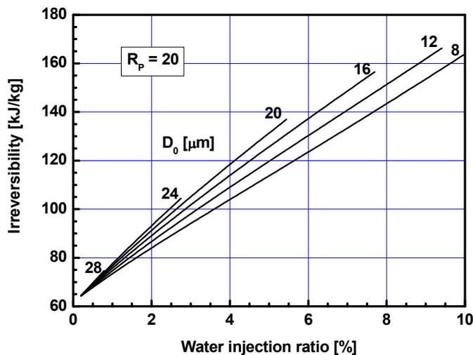
**Figure 8.** Effects of water injection ratio and initial droplet diameter on the ratio of inlet fogging irreversibility to total irreversibility at pressure ratio  $R_p = 20$ .
