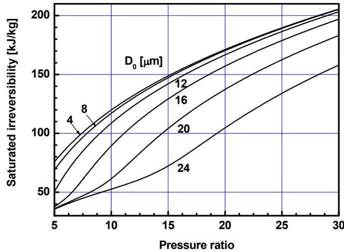
**Figure 12.** Effects of pressure ratio and initial droplet diameter on the ratio of inlet fogging irreversibility to total irreversibility at the saturated water injection ratio.
