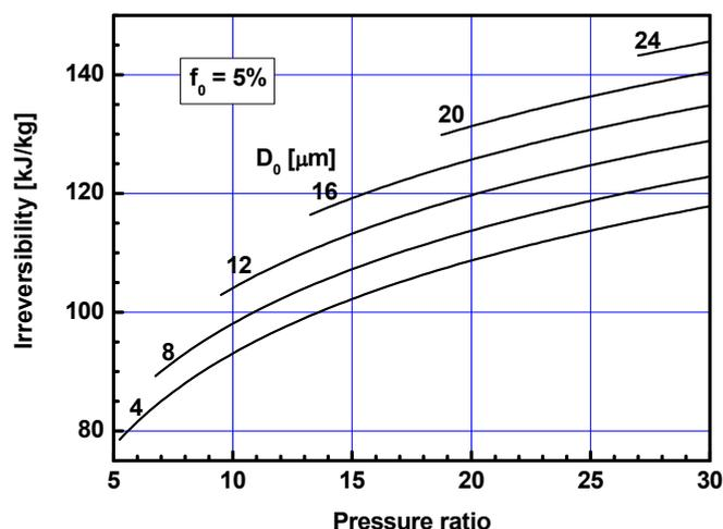
**Figure 4.** Effects of pressure ratio and initial droplet diameter on the ratio of inlet fogging irreversibility to total irreversibility at water injection ratio  $f_0 = 5\%$ .
