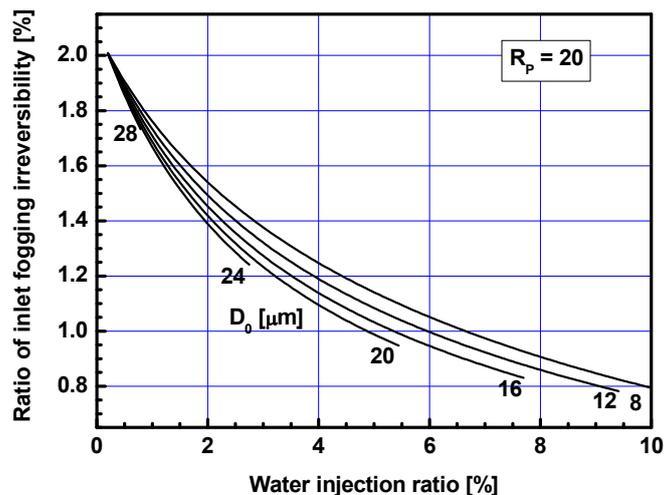
**Figure 9.** Effects of water injection ratio and initial droplet diameter on the exergy efficiency at pressure ratio  $R_p = 20$ .
