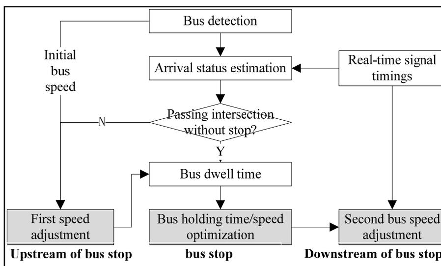
There are three steps for the optimization of dynamic bus speed and bus holding time for every detected bus. The functions of the three parts are introduced as follows:
