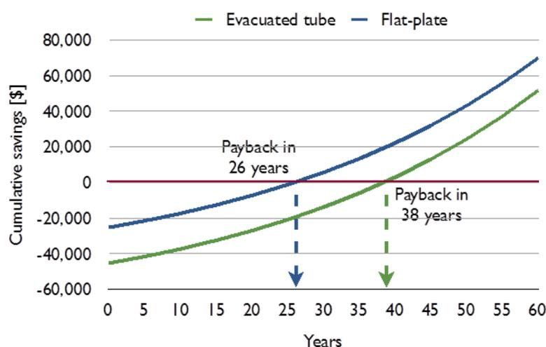
The improved payback period of the seasonal storage system was quite long, from 55 to 38 years for design alternative No.1 (depending on the economic scenario), and from 34 to 26 years for design alternative No.2. The only way to obtain a payback period under the 30-years life span of the system is to benefit from substantial incentives. These results are seen as the direct consequence of the high
