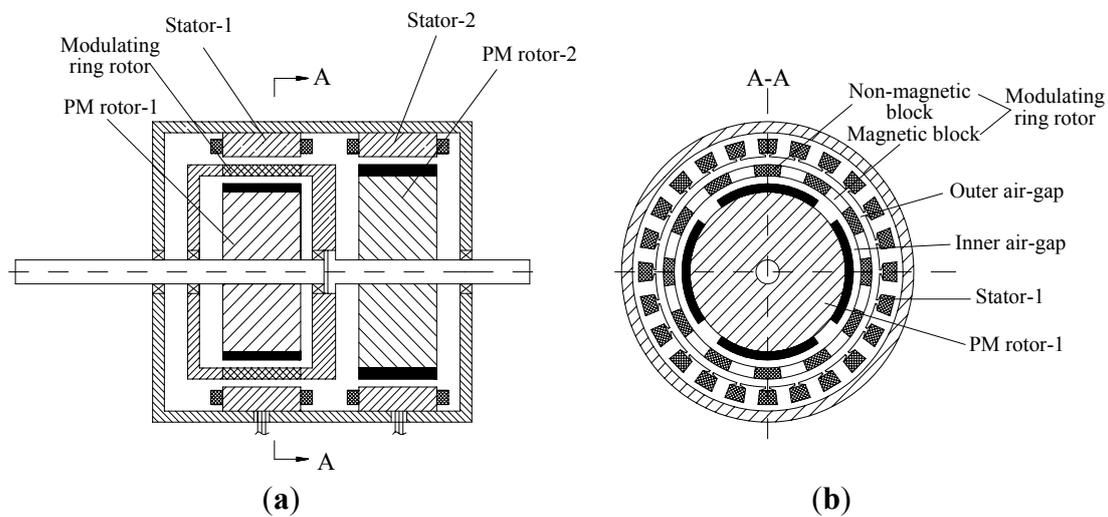
According to the operating principle of flux-modulated magnetic gear [14,15], the pole pair numbers of the PM rotor-1, the stator and magnetic blocks satisfies:
