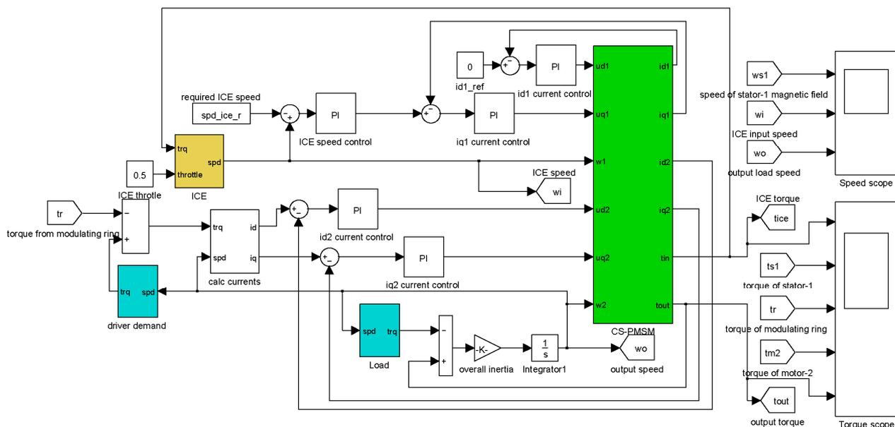
The pole pair numbers of PM rotor-1 and PM rotor-2 are 19 and 4, respectively, and the magnetic block number of modulating ring is 23. The output moment of inertia is considered, so the transient process of speed change can be observed. Vehicle air drag, rolling resistance and road grade are
