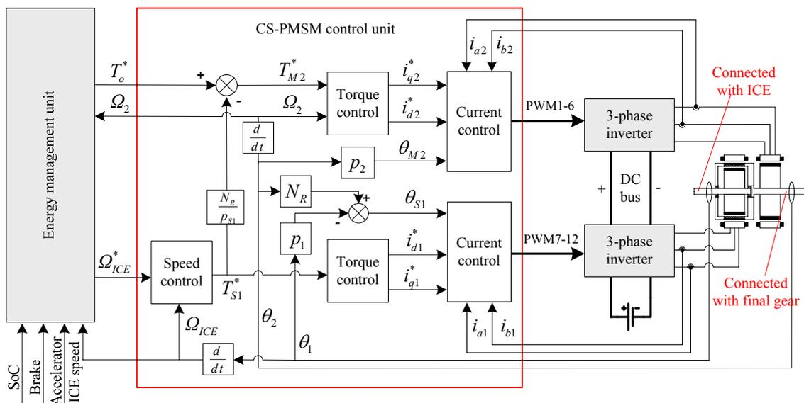
Two resolvers are installed for position feedback of the dual rotors, so the instantaneous electrical angular of the DRM can be calculated according to its operating principle. The two 6-switch inverters share the same DC bus. A DC-DC converter may be used to boost the low battery voltage for the inverters or buck the high DC link voltage for battery charge. This is useful for reducing the size of
