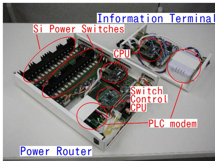
The terminal gathers information from both power sources and loads. The CPU decides the optimal combination of the source and the load according to the information on supply and demand of power. The information of the source-and-load pair is transferred to the power router via PLC.
