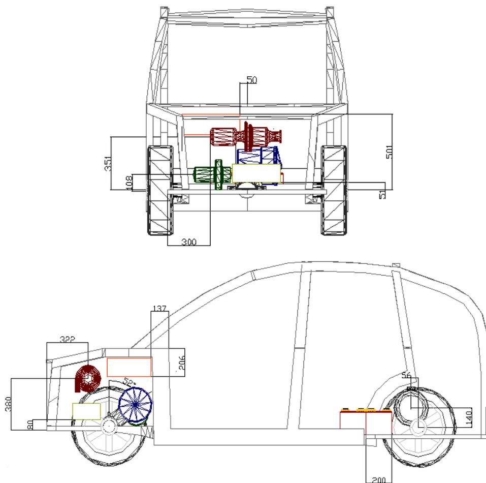
Figure 10. Weight distribution in the LETHE™ City Car configuration.
