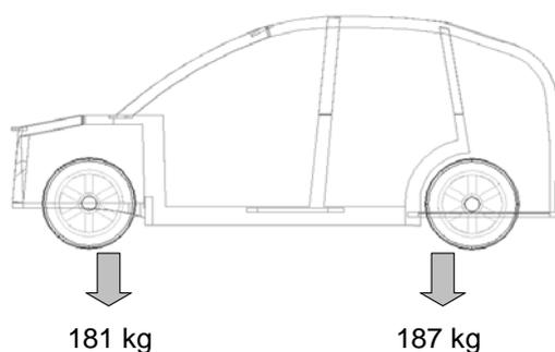
In spite of the presence of the second GT unit, all the parts can still be comfortably installed in the area available under the Audi A2 bonnet. The two turbo-gas units were placed centrally and staggered in order to leave enough space for the air vents and the various connection pipes. The weights were equally distributed on the two wheel axles. In spite of the fact that the parts were closer than in the previous solutions, the motor area is still easily accessed and ventilated.
