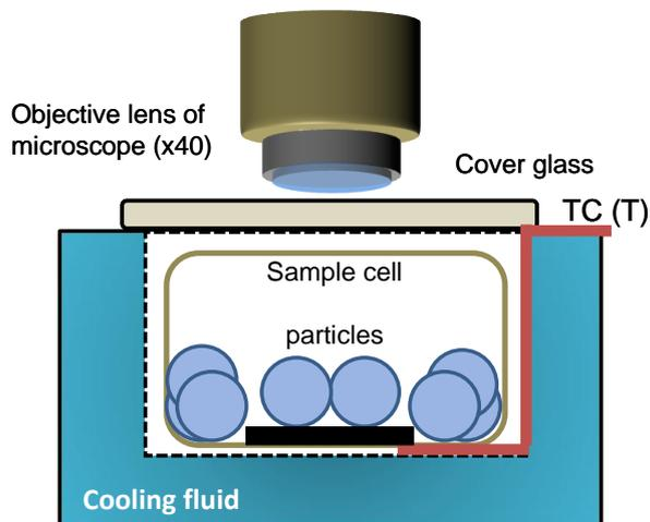
To validate the experimental procedure, the same experiments were carried out on pure ice particles. For experiments under the THF saturation condition, the particle samples were placed on the stage in the sample cell (black rectangle in Figure 8), which was immersed in a small amount of THF solution at the bottom of the cell instead of extra particles. The sample sizes used in the present study are summarized in Table 1.
