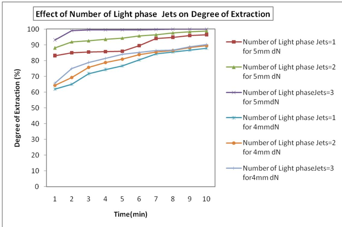
That is why the increase in degree of extraction with total operating time is not appreciable as the number of light phase jets increases. The degrees of extraction found were 87.9%, 89.6% and 90.2% for one, two and three light phase jets respectively. The force of the jet is decreased due to the static pressure applied by the pool of the heavy phase.
