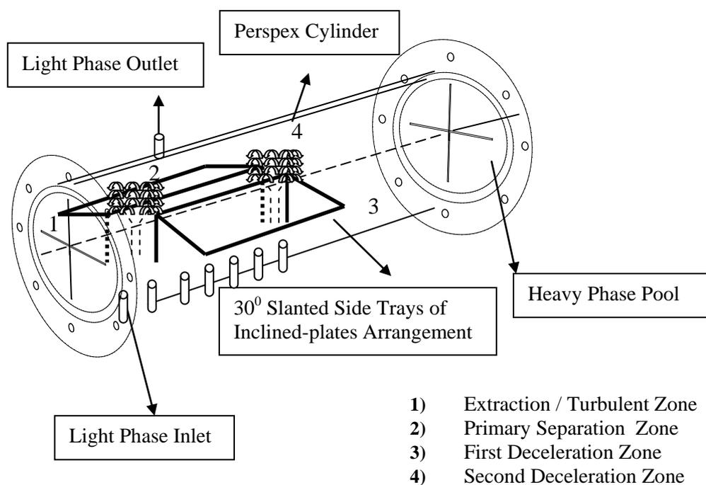
**Figure 5.** Motion of the coalesced films on the inclined plates while heavy phase falling back to the bottom of the vessel for further contact and re-entrainment by the jetted light phase.
