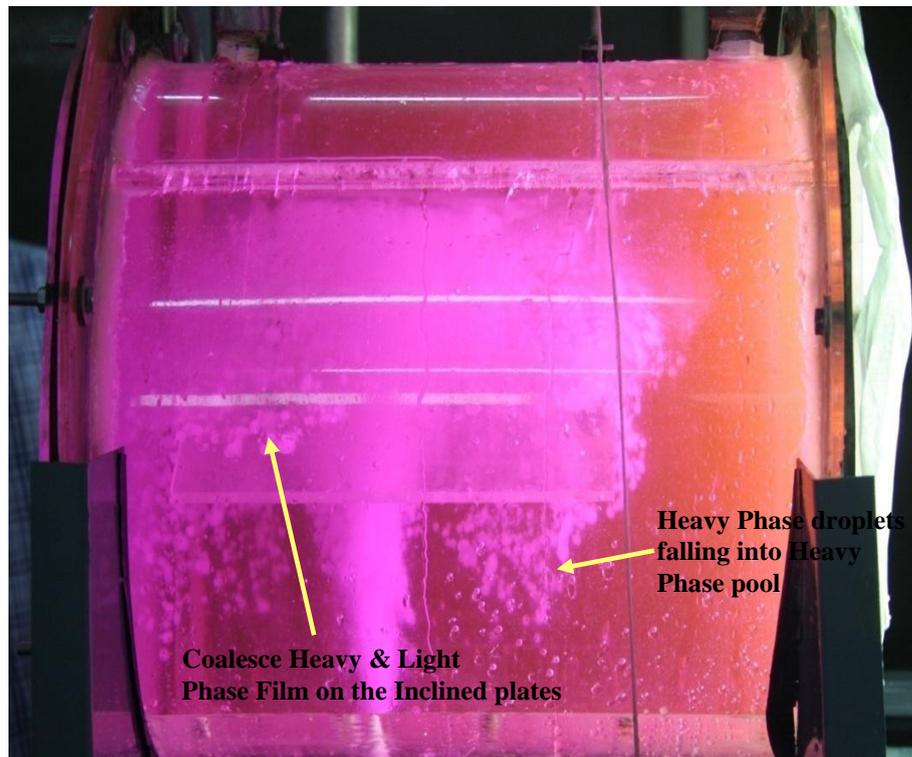
It has been found by Daood that 12.5 cm from the top cylindrical wall of the vessel is the optimum inclined plate position for both 4 mm and 5 mm diameter jets for the same system [36].
