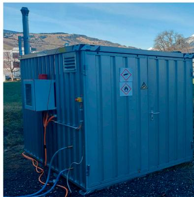
**Figure A1.** An outdoor container at OST used to test flammable refrigerants with the laboratory high-temperature heat pump.
