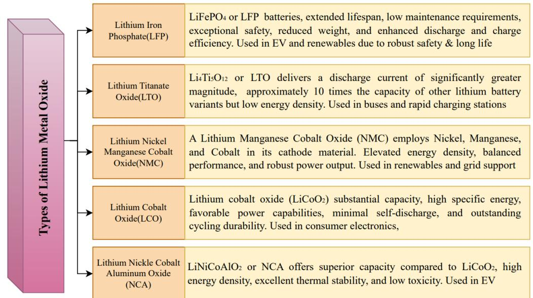
Figure 2. Different types of lithium metal oxides and key characteristics [15,16].
