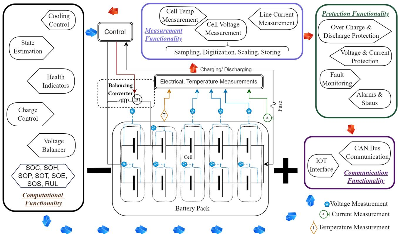
Figure 3. Battery management system (BMS).
