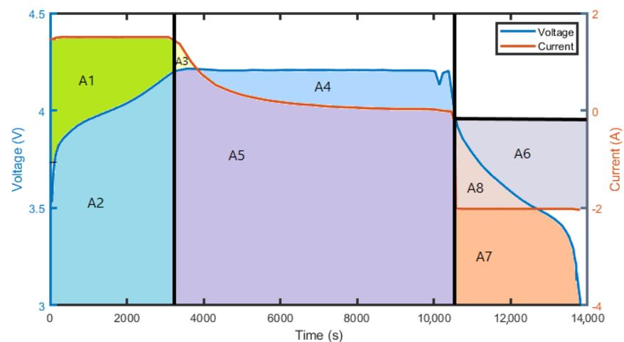
Figure 7. Voltage- and current-integral-based HIs.
