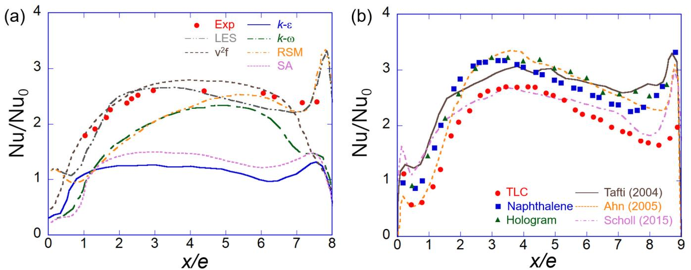
**Figure 3.** The local Nusselt number distribution on the channel wall between the ribs; (a) RANS data [12] ( $v^2f$  from [83]) compared to experiment [84]; (b) Three experiments [47,85,86] and three LES data [38,47,57]. SA: Spalart–Allmaras.
