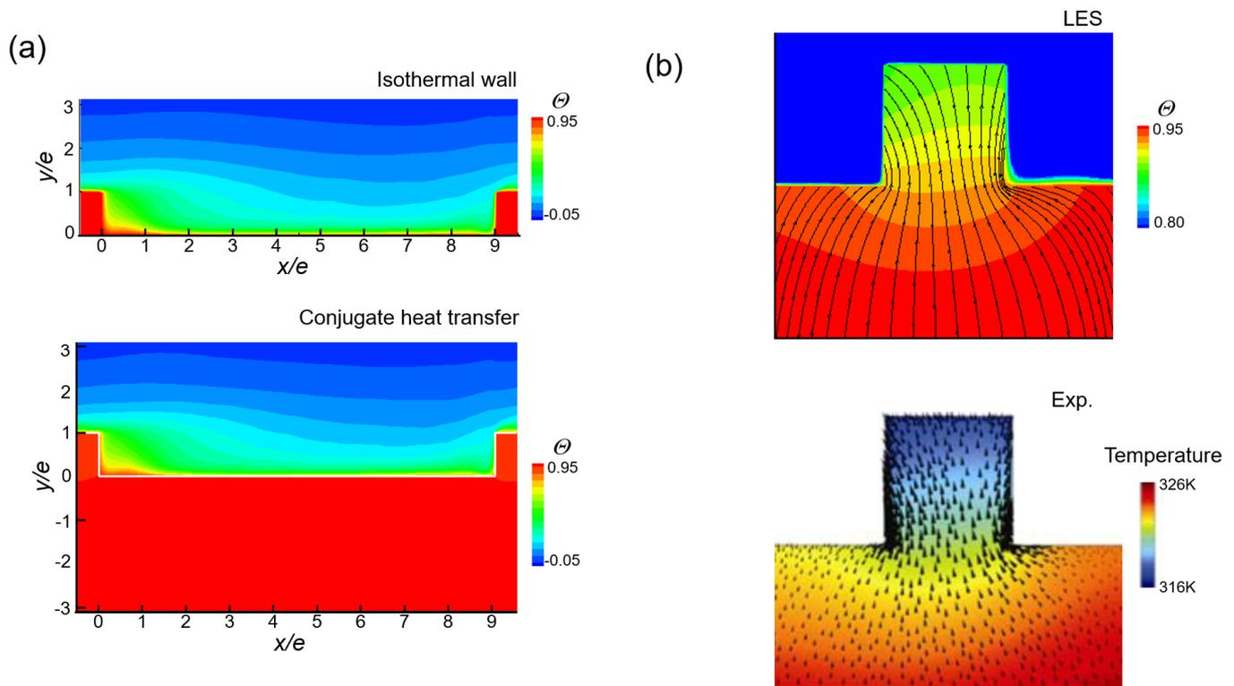
**Figure 7.** Thermal fields in a ribbed channel with a conducting wall [10]: (a) temperature contours in the  $xy$  plane; (b) the temperature around the rib.
