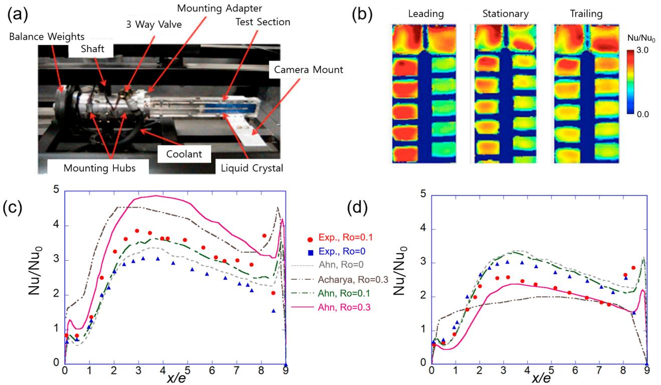
**Figure 9.** Heat transfer in the rotating ribbed channel: (a) A typical experimental setup [3]; (b) local heat transfer distributions [3]; (c) the local Nusselt number on the trailing wall; (d) the local Nusselt number on the leading wall.  $Ro$ : rotation number (LES data [48,50] compared to experiment [91]).
