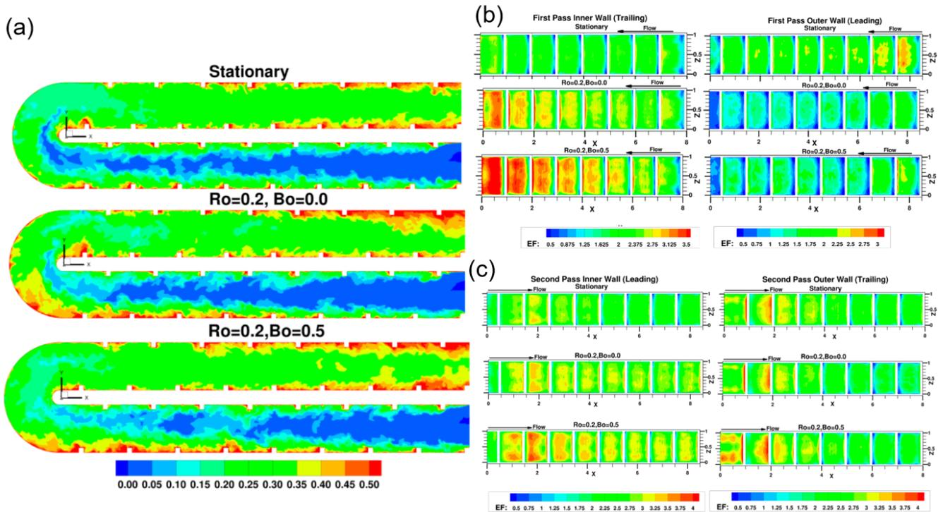
**Figure 10.** Large eddy simulation of heat transfer in a two-pass rotating ribbed duct [43]: (a) thermal fields in the channel; (b) heat transfer on the channel wall during the first pass; (c) heat transfer on the channel wall during the second pass.  $Bo$ : buoyancy number.
