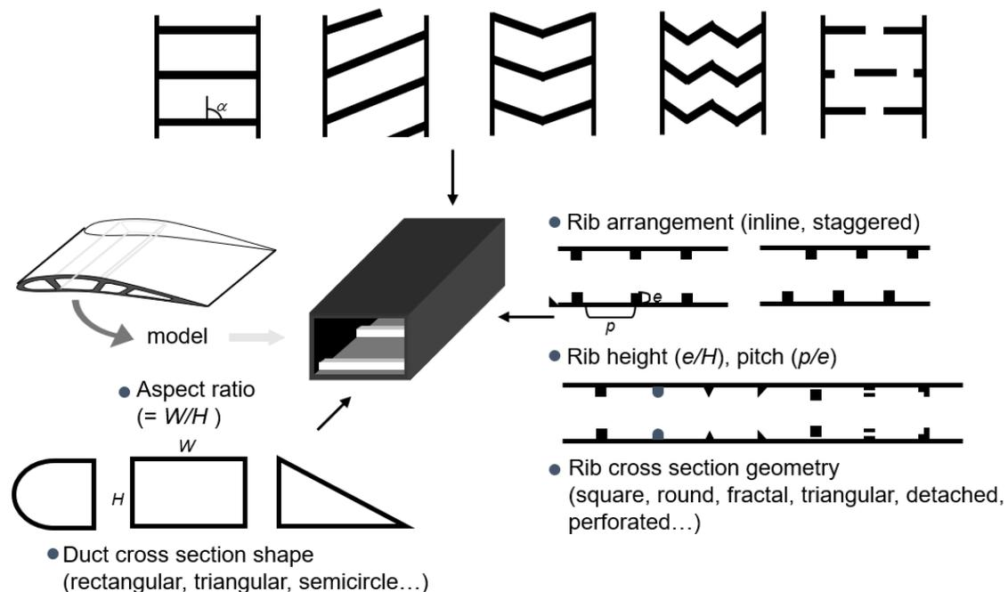
**Figure 11.** Geometrical shapes and variables affecting heat transfer in the internal cooling passage of a gas turbine.
