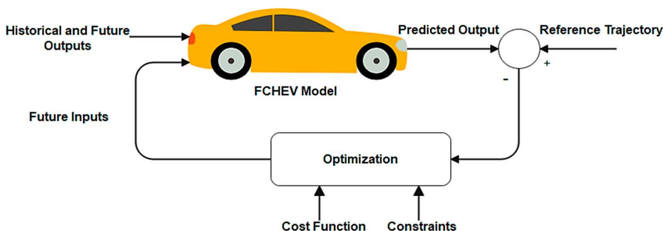
**Figure 10.** MPC flowchart for FCHEV.
