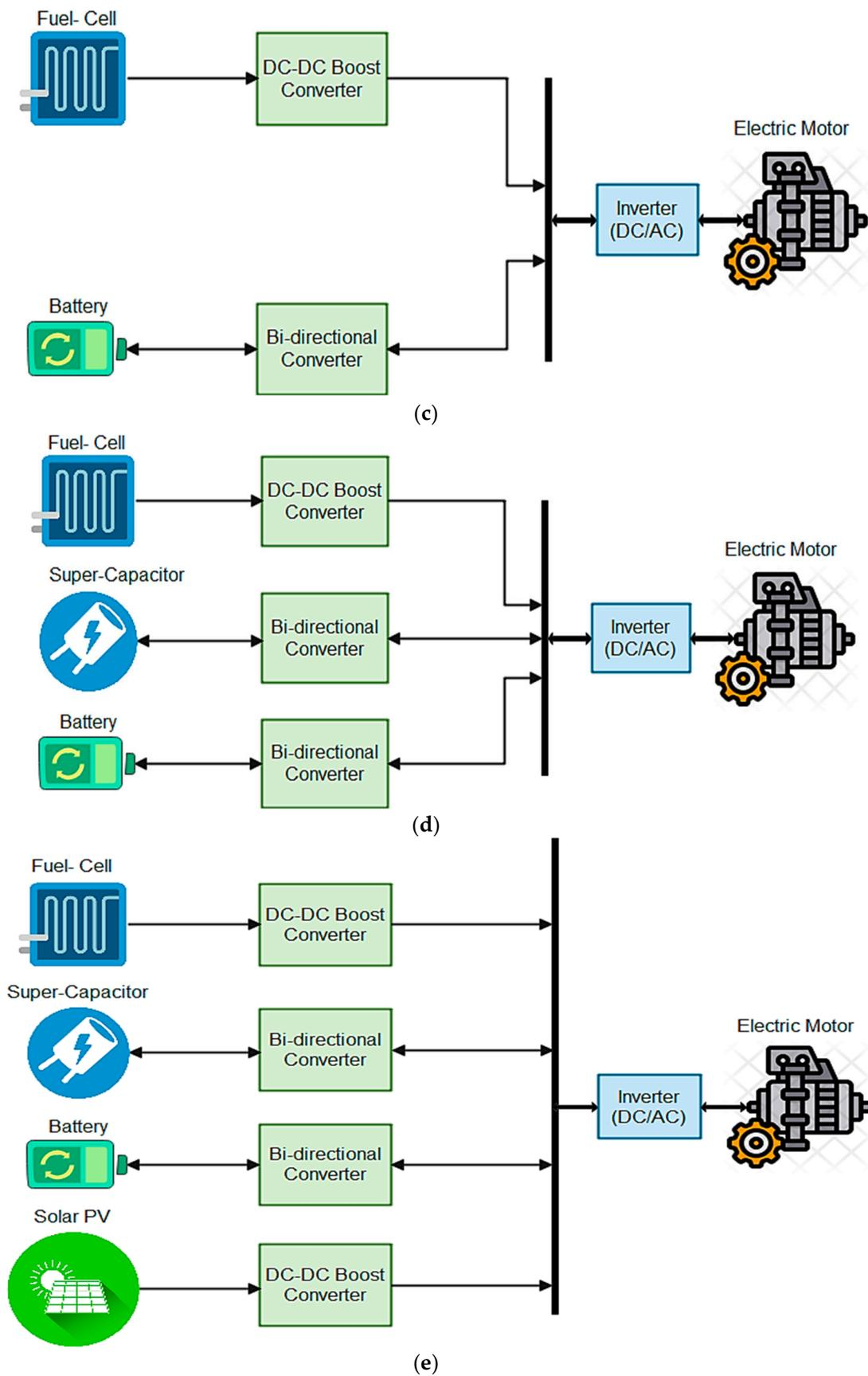
Figure 4. FCEV power source configurations: (a) FC only; (b) FC-SC; (c) FC-Battery; (d) FC-SC-Battery; (e) FC-SC-PV-Battery.
