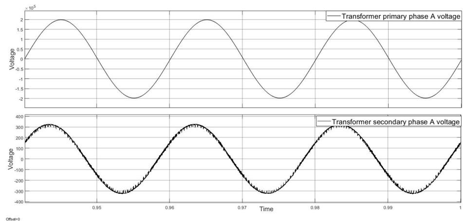
Figure 7. Transformer primary and secondary A phases voltage signals.
