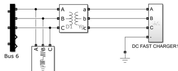
**Figure 2.** A 6-bus system EV charging station connection.
