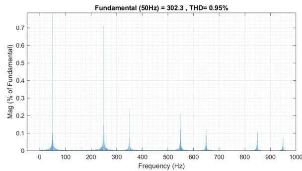
**Figure 15.** Transformer secondary/rectifier input voltage total harmonic distortion for three EV fast chargers.
