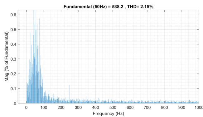
Figure 9. Transformer secondary/rectifier input current total harmonic distortion.
