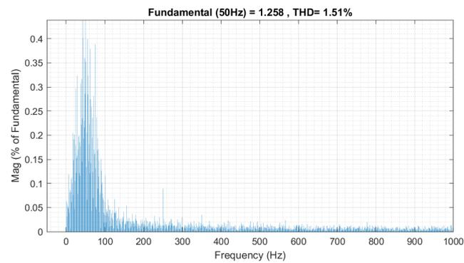
Figure 8. Transformer primary current total harmonic distortion.
