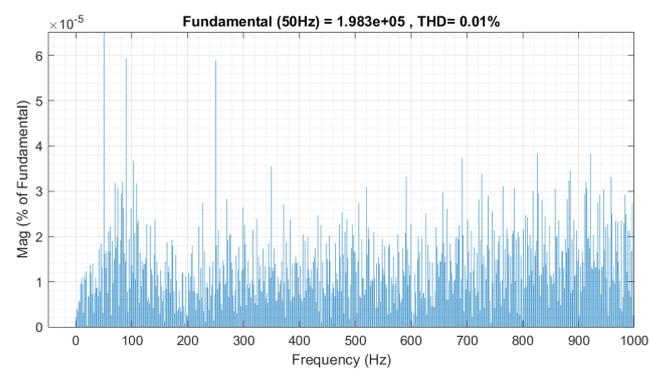
Figure 10. Transformer primary voltage total harmonic distortion.
