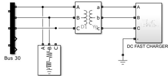
Figure 4. A 30-bus system EV charging station connection.
