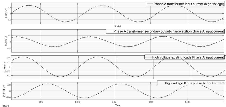
Figure 5. The 6-bus system EV charging station current signals.
