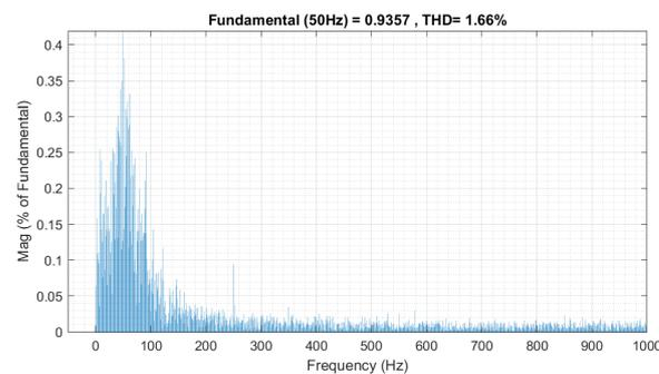
**Figure 12.** Transformer primary current total harmonic distortion for three EV fast chargers.
