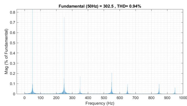
Figure 11. Transformer secondary/rectifier input voltage total harmonic distortion.
