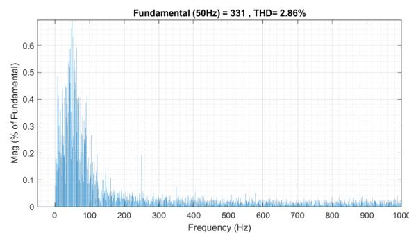
**Figure 13.** Transformer secondary/rectifier input current total harmonic distortion for three EV fast chargers.
