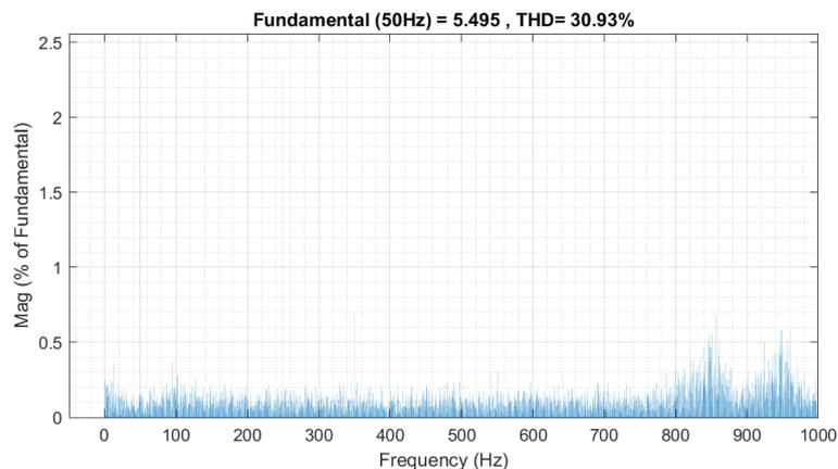
**Figure 18.** A 6-bus system current harmonic spectrum when SOC (state of charge) is 90%.
