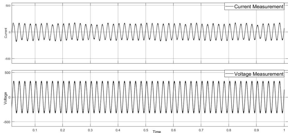
Figure 6. EV charging station rectifier input current and voltage signals.
