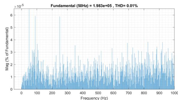
**Figure 14.** Transformer primary voltage total harmonic distortion for three EV fast chargers.
