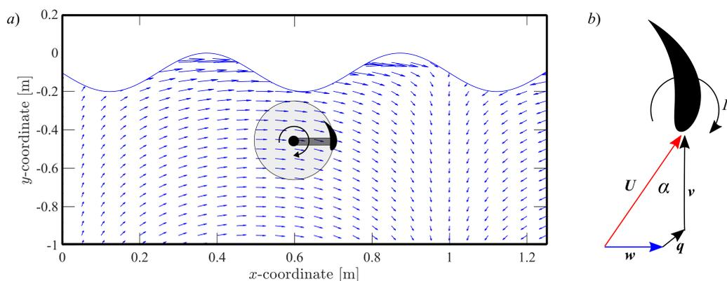
**Figure 7.** (a) Single foil wave cycloidal rotor beneath surface level and interacting with wave velocity field and (b) velocity triangle of the foil due to wave velocity component  $w$ , induced velocity due to the circulation of the foil and the memory effect on the free surface  $q$  and velocity component due to rotation of foil  $v$  [5,35].
