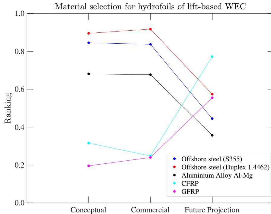
**Figure 9.** Rankings of materials for the hydrofoils of a lift-based WEC during three different design stages: conceptual, commercial and future projection stages.
