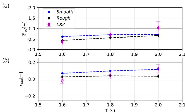
**Figure 8.** (a) Radial and (b) tangential force coefficient validation with simulated results for rough and smooth hydrofoils and compared versus experimental data [5].
