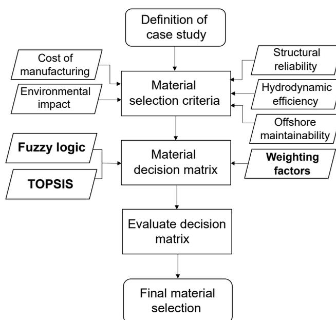
**Figure 1.** Flow chart illustrating the MCDM material selection framework, with fuzzy logic, TOPSIS and weighting factors highlighted in bold, as key elements of the decision matrix.
