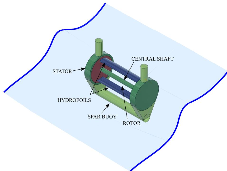
**Figure 2.** Floating lift-based WEC concept from LiftWEC project with horizontal spar buoy, two hydrofoils and a central shaft.
