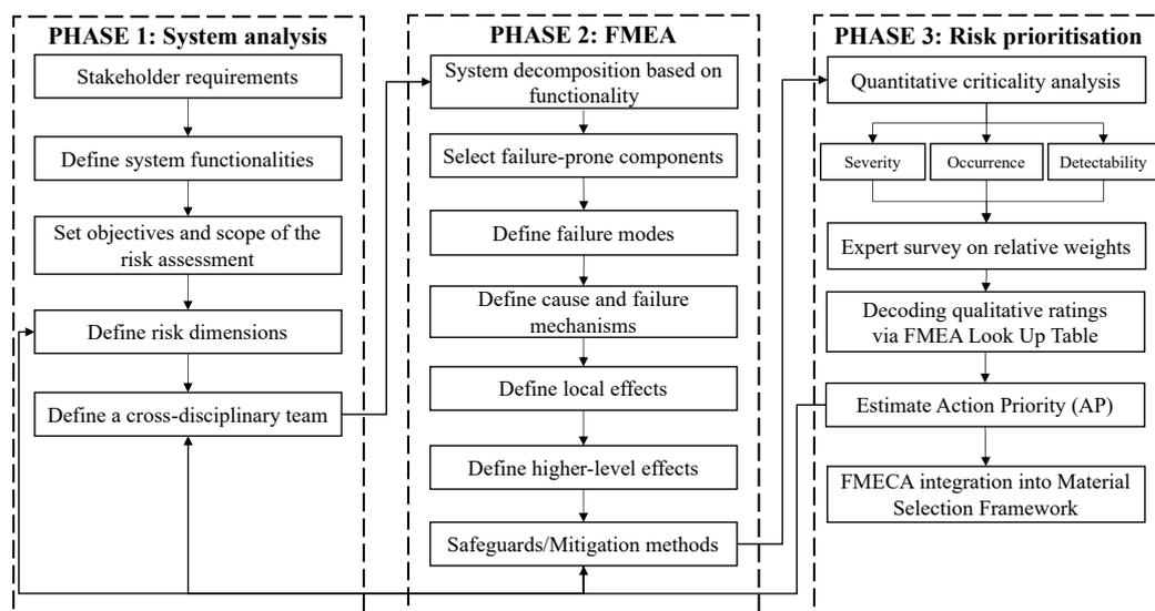
**Figure 6.** FMECA flowchart showing phase 1: System analysis, phase 2: FMEA and phase 3: Risk prioritisation.
