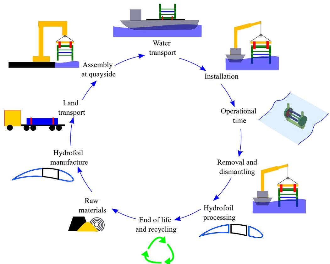
**Figure 4.** Material life cycle for lift-based wave energy converter.
