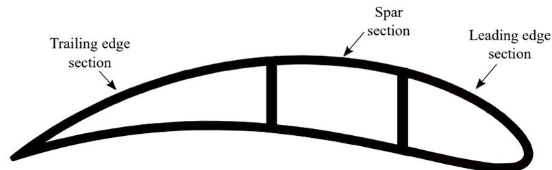
**Figure 3.** Curved hydrofoil cross-section for lift-based cycloidal rotor, showing the leading edge, spar and trailing edge sections.
