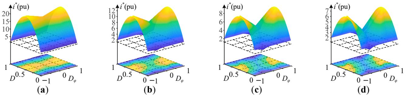
Figure 8. Current stress under the full operational area: (a)  $m = 0.1$ ; (b)  $m = 0.2$ ; (c)  $m = 0.3$ ; (d)  $m = 0.4$ .
