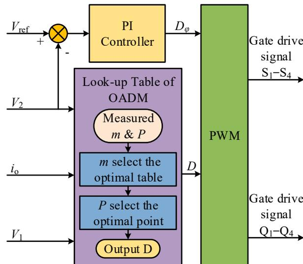
**Figure 11.** Overall control scheme of OADM.
