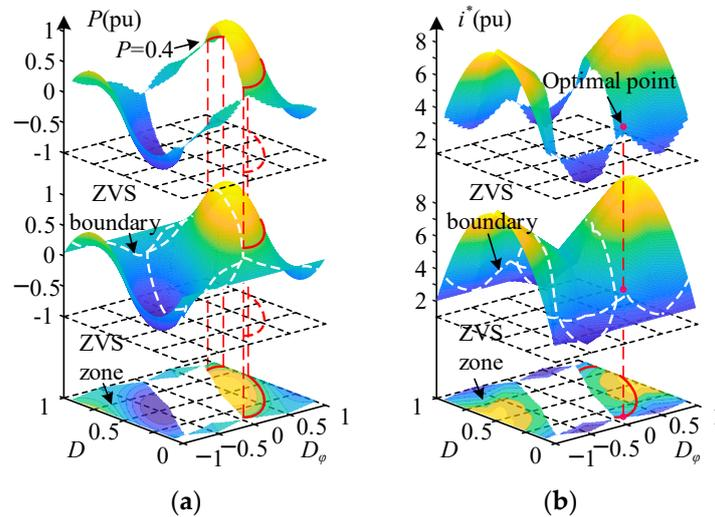
**Figure 10.** Optimization process of current stress with full ZVS: (a) equal power line with full ZVS; (b) optimal point.
