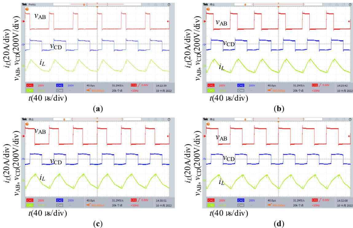
**Figure 13.** Waveforms of mode A with the same phase shift: (a)  $D = 0.2$  ( $P = 0.465$ ); (b)  $D = 0.3$  ( $P = 0.782$ ); (c)  $D = 0.4$  ( $P = 0.952$ ); (d)  $D = 0.5$  ( $P = 0.948$ ).
