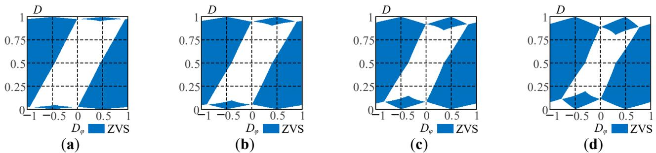
Figure 7. Range of ZVS under the full operational area: (a)  $m = 0.1$ ; (b)  $m = 0.2$ ; (c)  $m = 0.3$ ; (d)  $m = 0.4$ .
