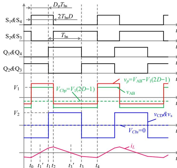
Figure 2. Typical waveforms of ADM.
