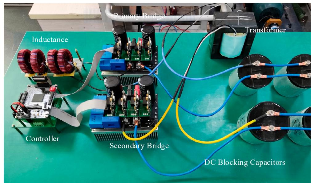
**Figure 12.** The prototype of a DAB converter with DC blocking capacitors.
