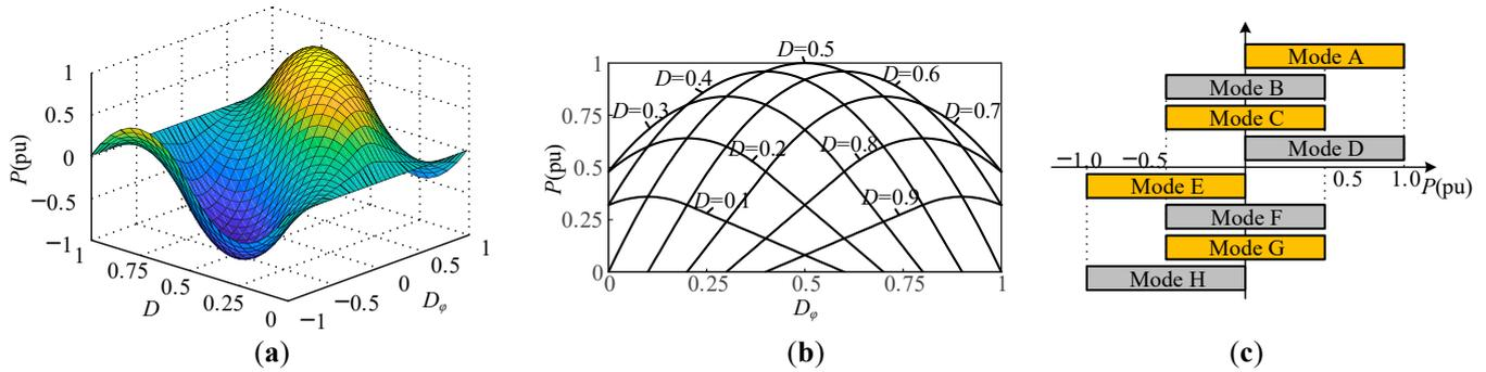
**Figure 6.** Transmission power: (a) 3D figure of  $D, D_\phi$ , and  $P$ ; (b)  $D_\phi \geq 0, P \geq 0$ , 2D figure of  $D, D_\phi$ , and  $P$ ; (c) transmission power range of each mode.
