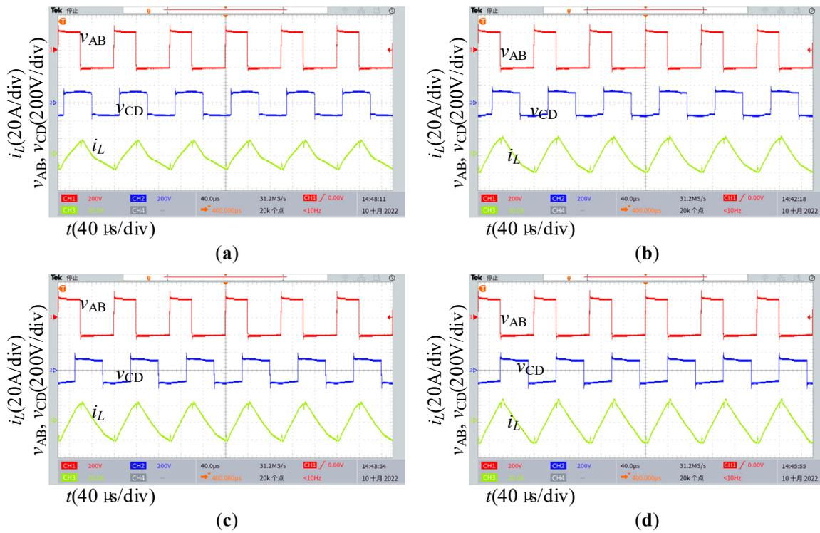
**Figure 14.** Waveforms of mode A with the same duty cycle: (a)  $D_\phi = 0.2$  ( $P = 0.776$ ); (b)  $D_\phi = 0.5$  ( $P = 0.914$ ); (c)  $D_\phi = 0.6$  ( $P = 0.784$ ); (d)  $D_\phi = 0.8$  ( $P = 0.287$ ).
