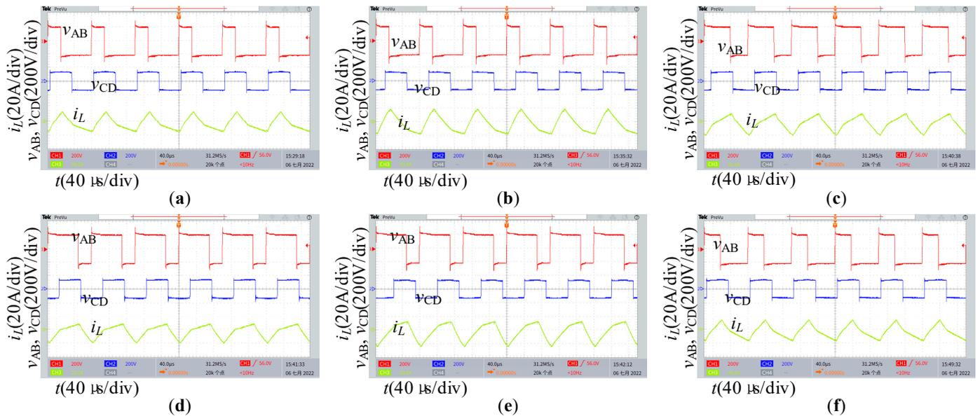
**Figure 15.** Waveforms of  $P = 0.76$ : (a)  $D = 0.31$ ,  $D_\phi = 0.09$ ; (b)  $D = 0.31$ ,  $D_\phi = 0.42$ ; (c)  $D = 0.61$ ,  $D_\phi = 0.31$ ; (d)  $D = 0.69$ ,  $D_\phi = 0.51$ ; (e)  $D = 0.71$ ,  $D_\phi = 0.82$ ; (f)  $D = 0.37$ ,  $D_\phi = 0.11$ .
