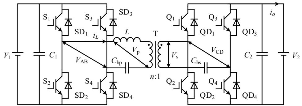
Figure 1. Topology of a DAB converter with DC blocking capacitors.
