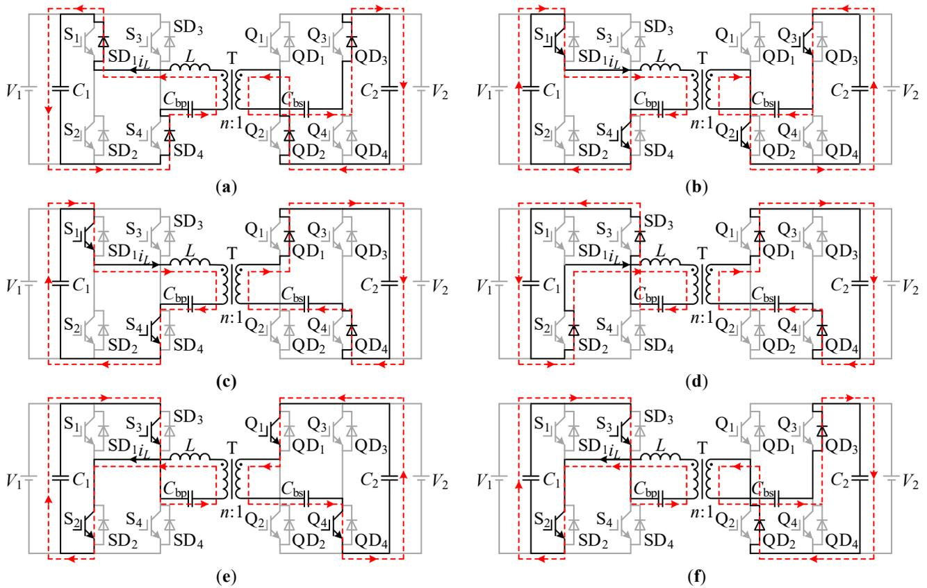
**Figure 5.** Equivalent circuits of stages in mode A: (a) stage 1; (b) stage 2; (c) stage 3; (d) stage 4; (e) stage 5; (f) stage 6.
