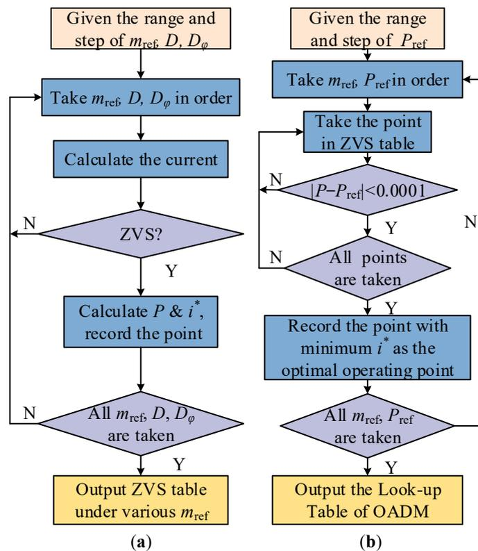
Figure 9. Flow chart of the off-line table-building procedure: (a) flow chart of the ZVS table; (b) flow chart of the optimal table.
