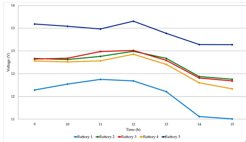
Figure 8. Favorable day: Cascading voltage behavior of the five batteries.
