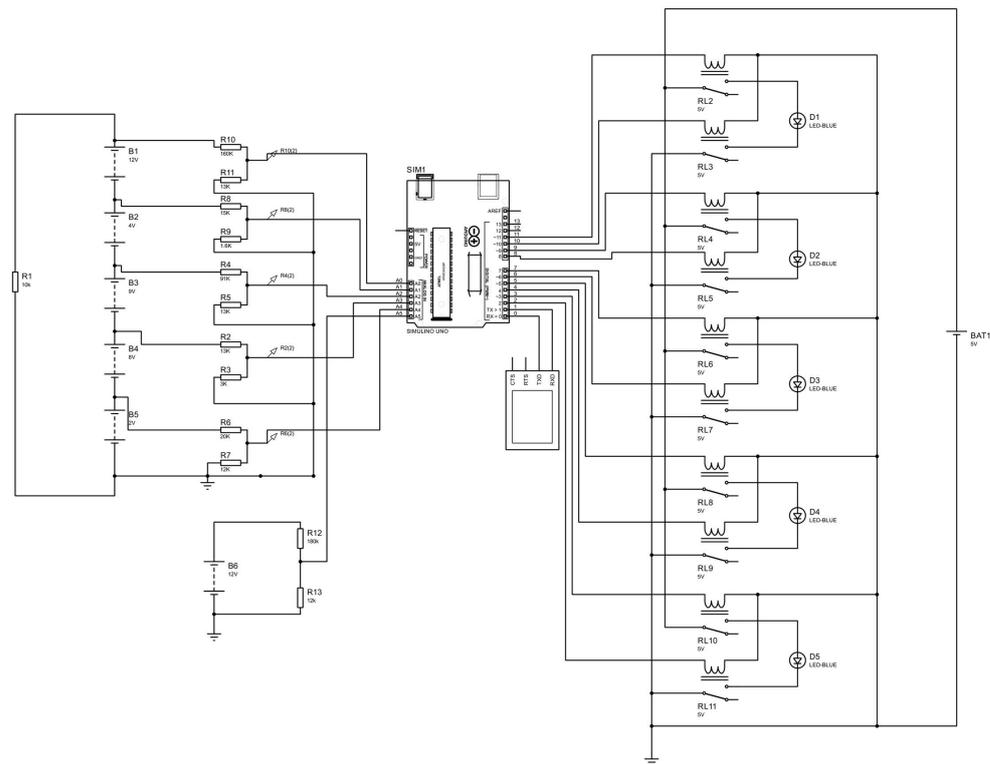
**Figure 2.** Load optimizing module diagram.
