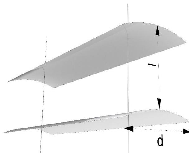
Figure 4. Representation of the slat width ( $d$ ) and spacing ( $l$ ).
