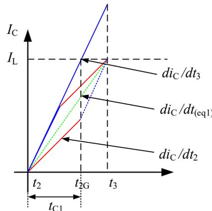
Figure 4. Equivalent schematic diagram of turn-on current rise rate.
