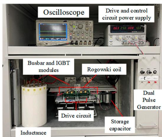
**Figure 13.** The experimental hardware circuit of the synchronous variable-amplitude drives method.
