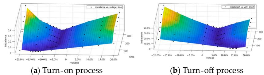
**Figure 10.** The three-dimensional relationship among drive control voltage, action time, and current unbalance degree in the turn-on and turn-off process. (The darker the color, the smaller the degree of current imbalance, while the lighter the color, the larger the degree of current imbalance.)
