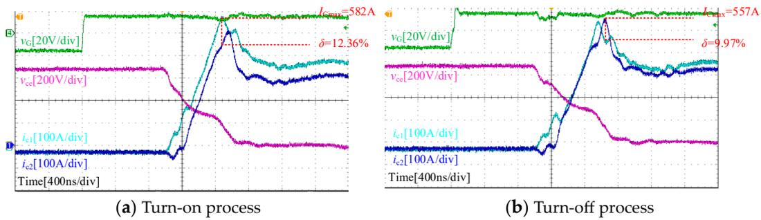
Figure 14. Waveform results of the parallel experiment of the two modules without compensation.
