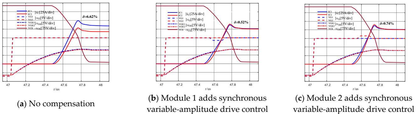
**Figure 8.** Comparison pre- and post-sync amplitude drive control in turn-on process.
