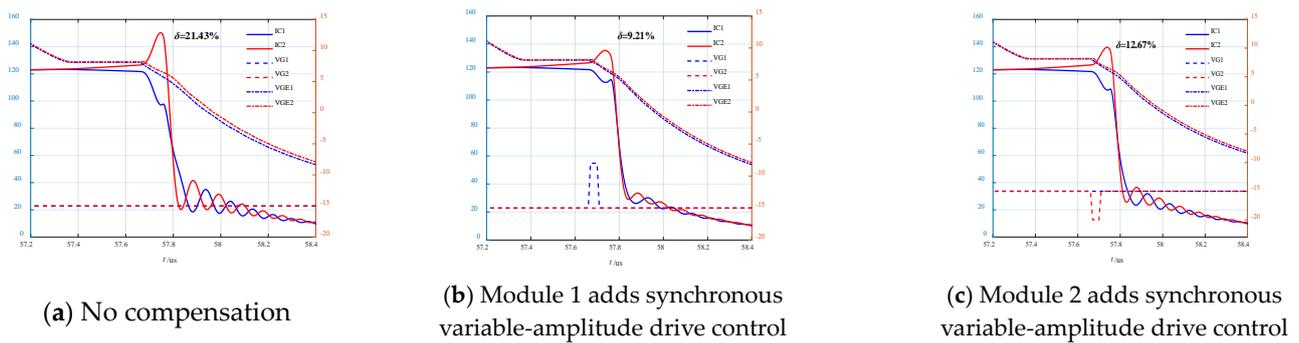
**Figure 9.** Comparison pre- and post-sync amplitude drive control in turn-off process.
