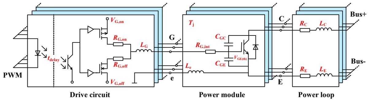
**Figure 1.** Circuit diagram of the parallel IGBT application circuit diagram including characteristic parameters affecting current sharing.
