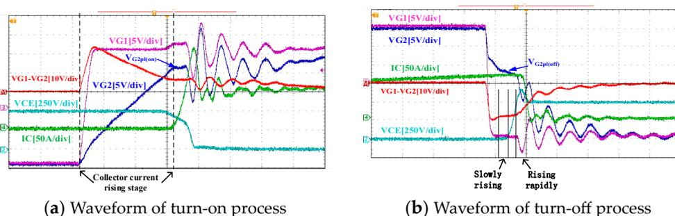
Figure 12. Experimental waveform of characteristic parameter extraction of IGBT module.
