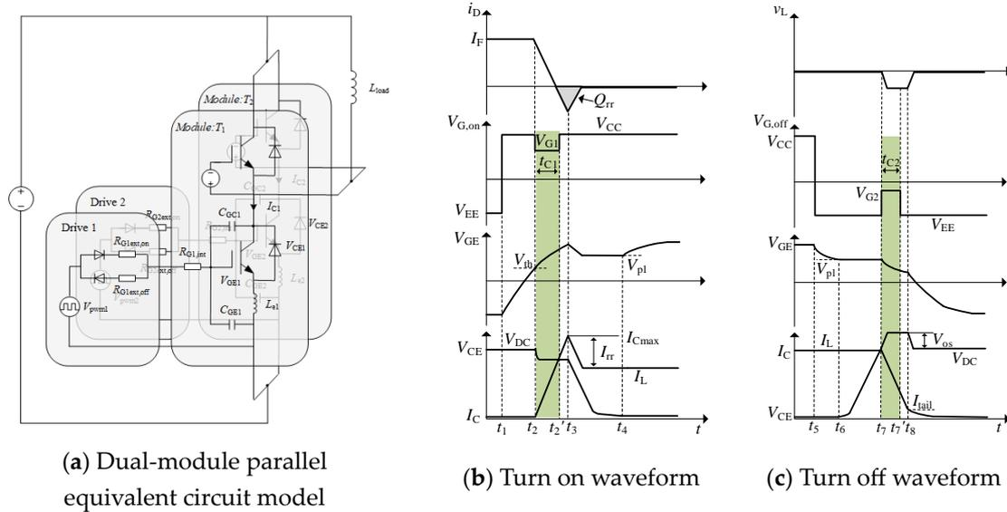
Figure 3. Dual-module parallel equivalent circuit model and process waveform.
