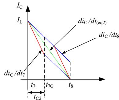
Figure 5. Equivalent schematic diagram of turn-off current rise rate.
