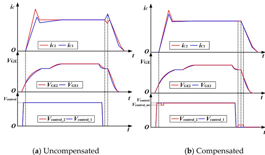
**Figure 2.** The principle of synchronous variable-amplitude driving method.
