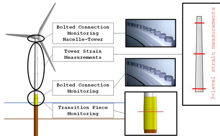
**Figure 7.** Scheme of the generic locations of monitoring system implementation for stress damage accumulation, bolted connection and grout monitoring.
