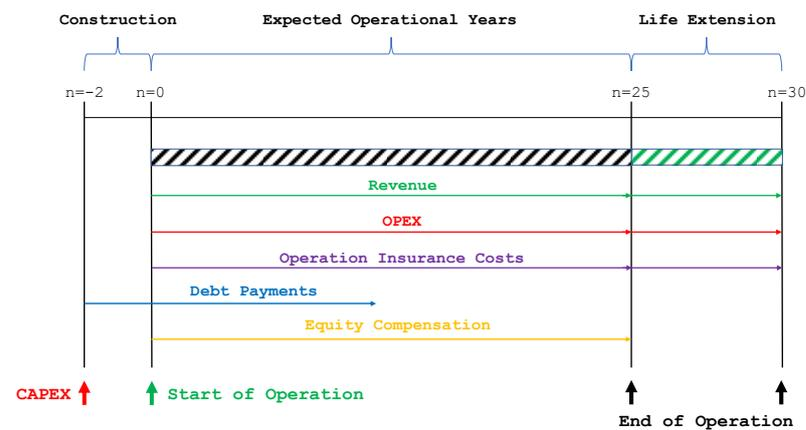
**Figure 13.** Framework of the cash-flow model developed, which considers three main life-cycle stages: construction, operation, and life extension.
