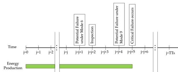
**Figure 9.** Flow of events over time for a turbine without SHMs. Adapted with permission from Ref. [56]. 2022, Elsevier.
