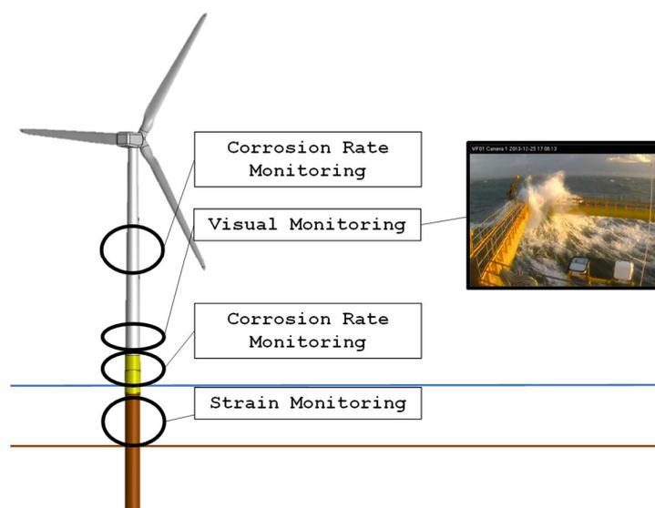
**Figure 8.** Scheme of the generic locations of monitoring system implementation for surveillance, corrosion monitoring and stress damage accumulation for the monopile.
