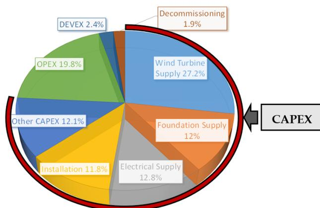
**Figure 2.** Cost Breakdown for Offshore Wind Levelized Cost of Energy. Data collected and adapted from NREL, The Crown Estate and TKI Wind op Zee [20–22].
