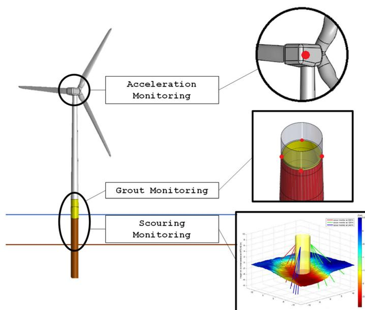
**Figure 6.** Scheme of the generic locations of monitoring system implementation for grout, scouring, and tower dynamics.
