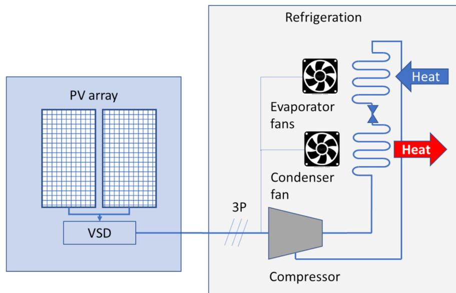
**Figure 3.** Basic electrical architecture for a solar-powered cold storage unit.
