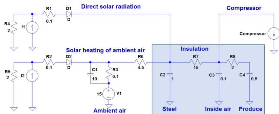
Figure 20. The dynamic thermal behavior of the cold storage modelled using an electrical equivalent circuit.
