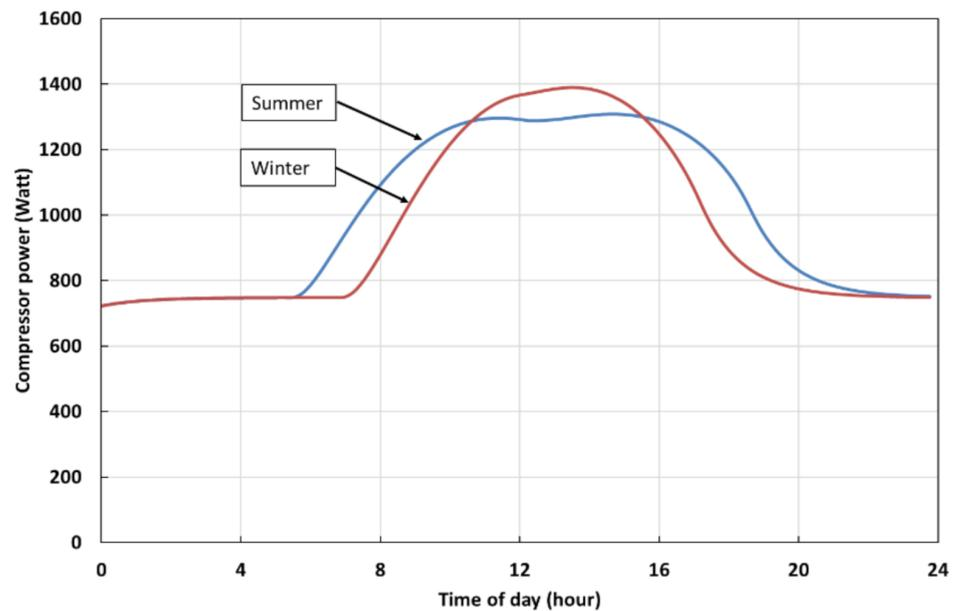
**Figure 15.** Compressor thermal power required to keep the cold storage temperature at 5 °C in mid-summer and mid-winter for a cold storage container orientated with the container face wall, normal to east, with all the container walls shaded.
