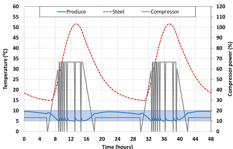
Figure 23. Produce temperature with a 66% increase in the insulation properties of the insulation layer.
