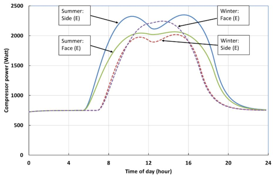
**Figure 14.** Compressor power required to maintain the cold storage at 5 °C for orthogonal container orientations in mid-summer and mid-winter. Side (E) indicates the container side wall normal to the east, Side (W) indicates the container side wall normal to the west, Face (N) indicates the container face wall normal to the north, Face (S) indicates the container face normal to the south, and Roof indicates the roof wall of the container, which is normal to up.
