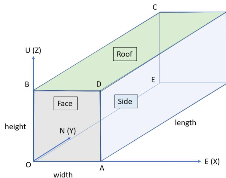
**Figure 5.** Cold storage container orientation definitions.
