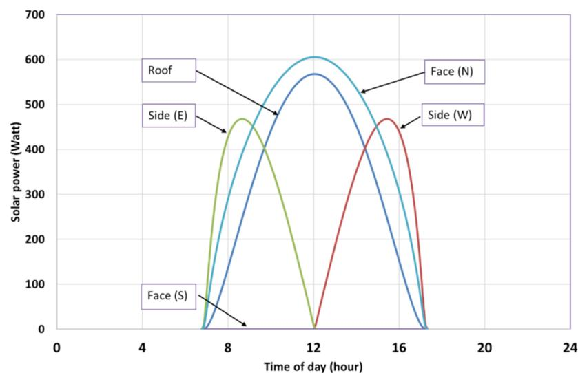
**Figure 7.** Solar radiation incident on the walls of the container over a winter's day. Side (E) indicates the container side wall normal to the east, Side (W) indicates the container side wall normal to the west, Face (N) indicates the container face wall normal to the north, Face (S) indicates the container face normal to the south, and Roof indicates the roof wall of the container, which is normal to up.
