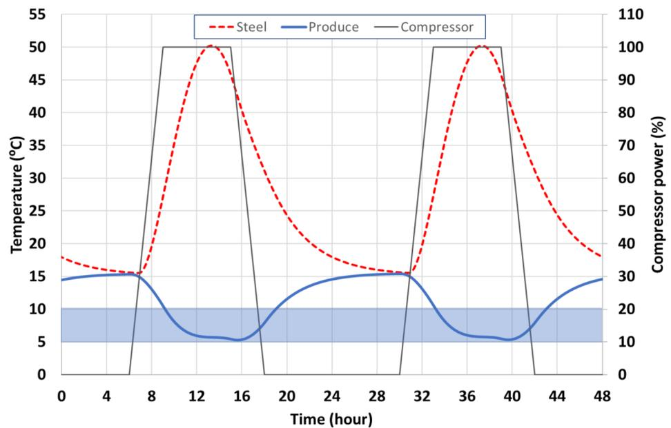
Figure 21. Produce temperature over a period of 48 h.
