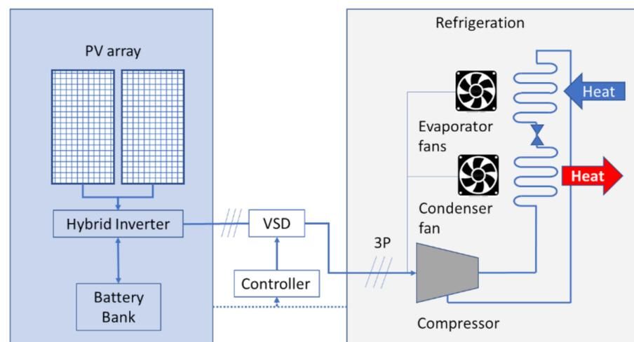
**Figure 4.** Advanced electrical architecture for a solar-powered cold storage unit.
