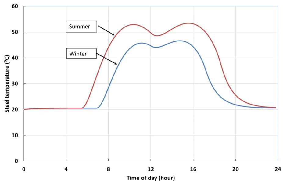
**Figure 9.** Steel container wall temperature for mid-summer and mid-winter.
