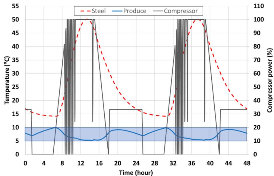
Figure 22. Produce temperature when running the compressor for an additional 7 h at night at a 33% power level.
