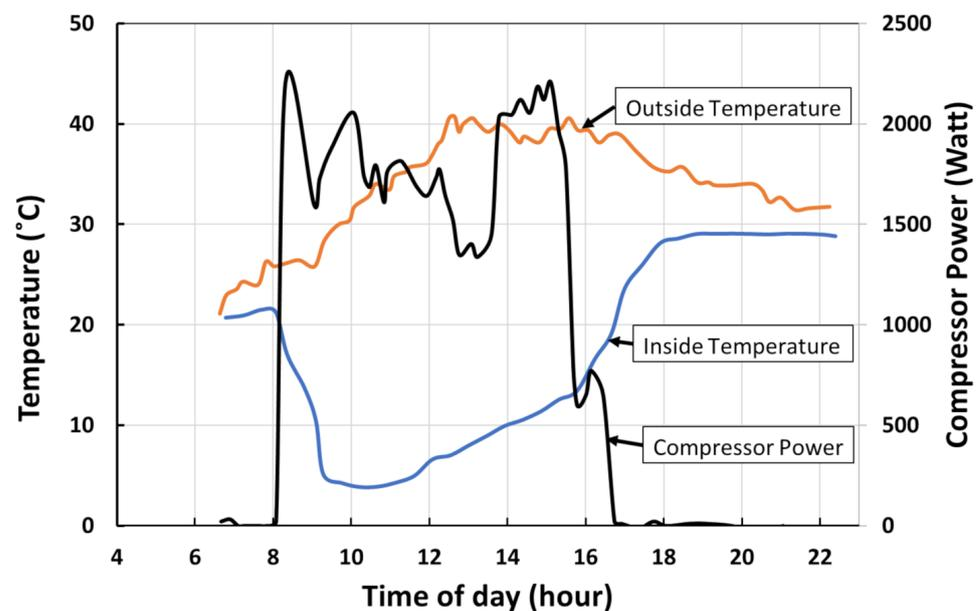
**Figure 2.** Gwakwani cold storage. Inside temperature, outside temperature, and compressor power consumption as measured on 4 December 2018.
