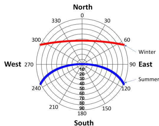
**Figure 16.** The Sun's elevation and azimuth angles during winter and summer for a solar PV installation at a 23.5° S latitude.
