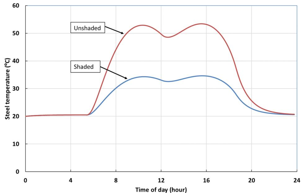
**Figure 10.** Container steel wall temperature in mid-summer shaded by the solar array mounted on top of the container vs. unshaded, where the solar panel array is mounted away from the container.
