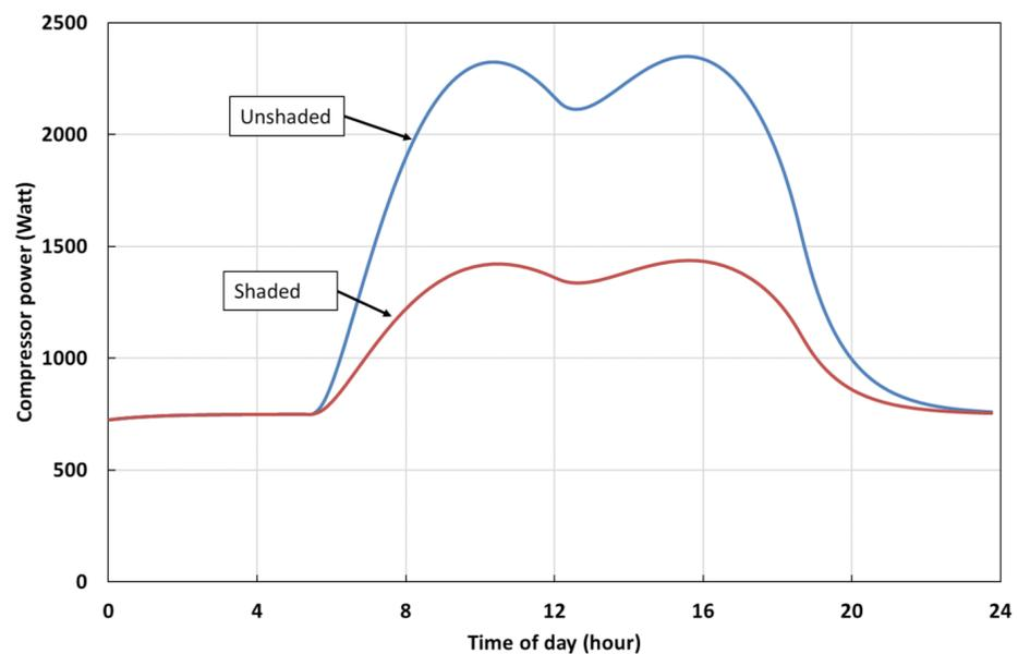
**Figure 11.** Compressor power required to maintain a constant 5 °C temperature inside the cold storage unit. Shaded by the solar array vs. unshaded container.
