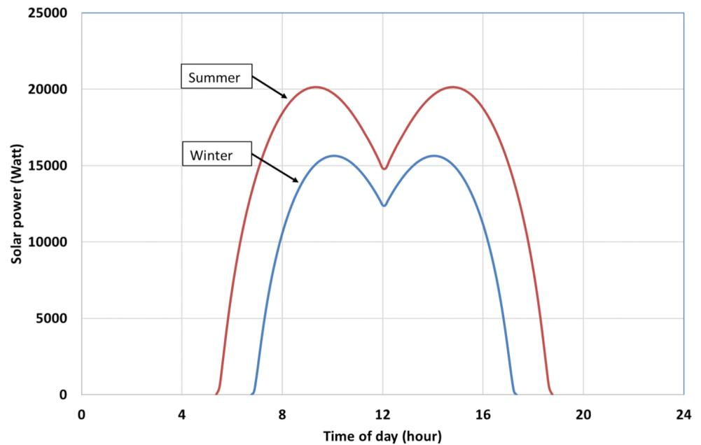
**Figure 8.** Total incident solar radiation on the container walls for mid-summer and mid-winter.
