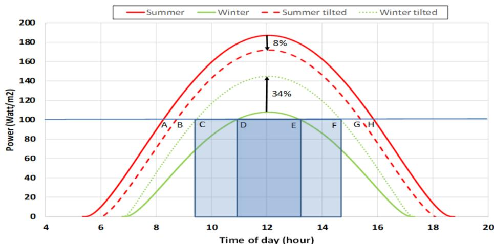
Figure 18. Available electrical power per unit of installed PV panels for a flat-mounted PV array versus a 23.5° northward-tilted PV array.
