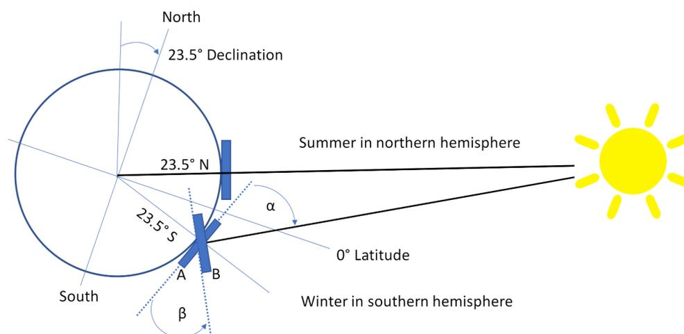
**Figure 17.** Solar incidence angle on a PV array in winter conditions, where the PV array is in the southern hemisphere and the Sun's orbit is in the northern hemisphere. (A) Local horizontally mounted PV array. (B) Locally tilt-mounted PV array.
