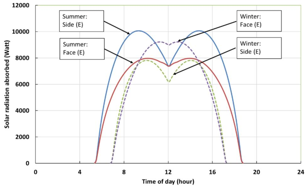
**Figure 13.** Solar radiation absorbed by the container in mid-summer and mid-winter for orthogonal orientations. Side (E) indicates the container side wall normal to the east, Side (W) indicates the container side wall normal to the west, Face (N) indicates the container face wall normal to the north, Face (S) indicates the container face normal to the south, and Roof indicates the roof wall of the container, which is normal to up.
