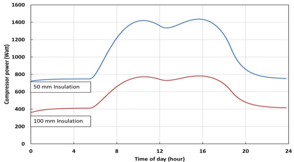
**Figure 12.** Required compressor thermal power for insulation materials 50 mm thick and 100 mm thick in summer with a shaded container.
