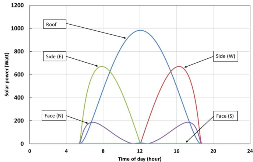
**Figure 6.** Solar radiation incident on the walls of the container over a summer's day. Side (E) indicates the container side wall normal to the east, Side (W) indicates the container side wall normal to the west, Face (N) indicates the container face wall normal to the north, Face (S) indicates the container face normal to the south, and Roof indicates the roof wall of the container, which is normal to up.
