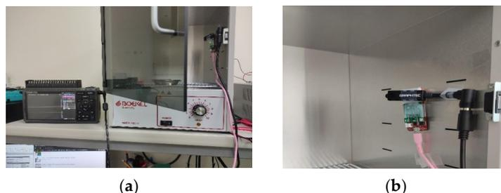
**Figure 10.** Calibration process of wireless climate sensor node: (a) measurement setup, (b) sensor node placement in a controllable test chamber.
