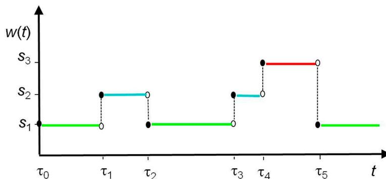
**Figure 11.** Example of the implementation of the process:  $\{U(t) : t \in T\}$  of a marine diesel main engine; (ME):  $\{U(t) : t \in T\}$ —process of state of repair;  $t$ —service life;  $s_1$ —full effective operability;  $s_2$ —partial operability;  $s_3$ —inoperability. Periods of time during which the use of the PTO/PTI system is justified.
