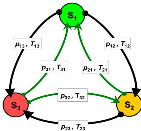
**Figure 10.** Ship’s main engine state change graph:  $s_1$ —full effective operability,  $s_2$ —partial operability,  $s_3$ —inoperability.  $p_{ij}$ —probability of process transition from  $s_i$  to  $s_j$ ,  $T_{ij}$ —duration of  $s_i$  provided that process transition to  $s_j$ ,  $i, j = 1, 2, 3$ .
