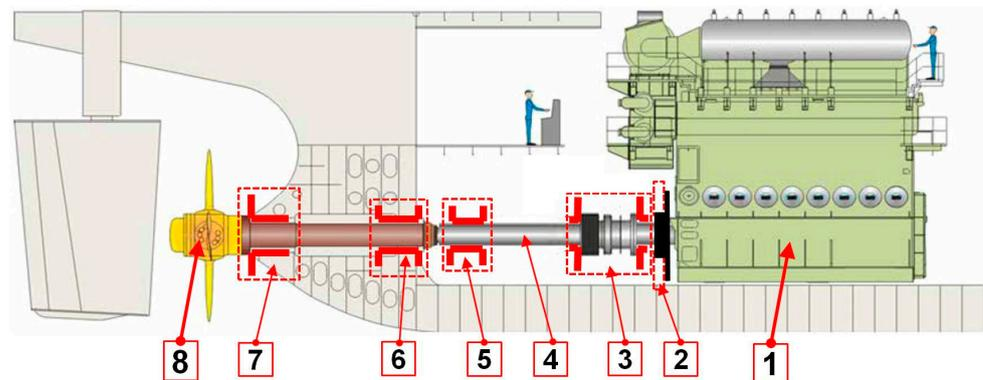
**Figure 2.** Sample diagram of the main propulsion system of the ship: 1—marine low-speed, two-stroke internal combustion main engine (ME), winged and slow-running; 2—non-disconnectable hydraulic coupling; 3—thrust bearing; 4—intermediate shaft; 5—bearing of intermediate shaft; 6—bearing of screw shaft; 7—scabbard of screw shaft; 8—fixed pitch propeller (own elaboration using MAN BW drive drawing [30]).
