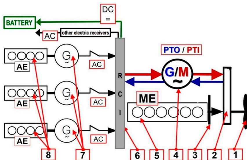
**Figure 1.** Example of the main propulsion system of the vessel: 1. Unregulated pitch drive screw propeller (fixed pitch propellers—FPP); 2. Electricity generator gearbox; 3. Clutch disconnecter; 4. Shafted alternator (PTO/PTI); 5. Marine low-speed, two-stroke main engine (ME); 6. RCI main power unit (AC/DC rectifier, AC/AC converter, DC/AC inverter); 7. Auxiliary engine (AE)—driven generators (G); 8. Auxiliary engine (AE) driving generators of ship power plants.
