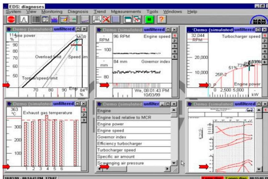
**Figure 7.** Complicated graphs of mathematical dependencies (at the level of higher mathematics, e.g., nonlinear functions) showing trends in changes of engine condition, on the basis of analysis of data provided by sensors placed on the engine, requiring [48].
