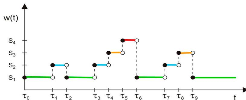
Figure 9. Example of the implementation of the  $\{W(t): t \in T\}$  process of a compression ignition engine:  $\{W(t): t \in T\}$ —process of state changes;  $t$ —operating time;  $s_1$ —full serviceability;  $s_2$ —incomplete serviceability;  $s_3$ —partial serviceability;  $s_4$ —unsuitable state; periods of time during which the use of a PTO/PTI system is justified.
