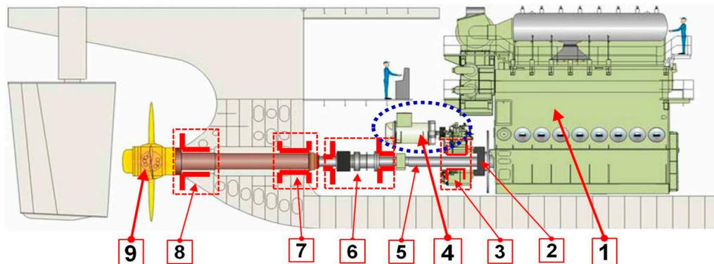
**Figure 3.** Example of ship’s main propulsion with shaft generator and PTO/PTI system: 1—marine low-speed, two-stroke diesel engine—main engine (ME); 2—hydraulic separable coupling; 3—shaft generator gear; 4—shaft generator (PTO/PTI); 5—intermediate shaft; 6—thrust bearing of intermediate shaft; 7—bearing of screw shaft; 8—stern tube; 9—fixed pitch propeller (own elaboration using MAN drawing [30]).
