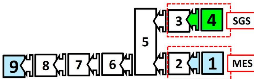
**Figure 4.** Scheme of main propulsion of the ship with shaft generator and PTO/PTI system: 1—two-stroke main motor; 2—hydraulic coupling; 3—shaft generator gear; 4—shaft generator (PTO/PTI); 5—intermediate shaft; 6—thrust bearing of intermediate shaft; 7—bearing of screw shaft; 8—stern tube; 9.—fixed pitch propeller; SGS—shaft generator systems; MES—main engine set (own elaboration).
