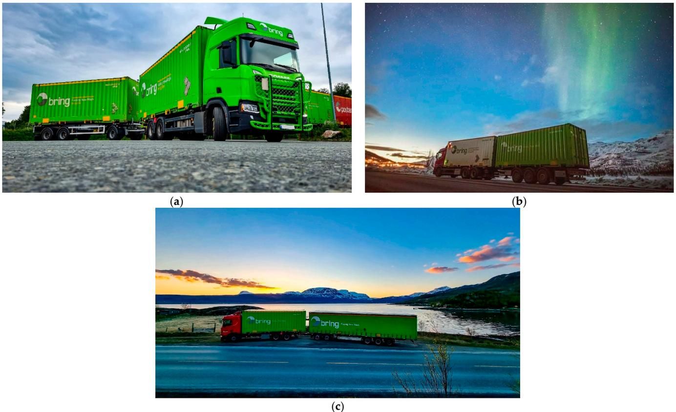
**Figure 1.** Truck + trailer with steered axle (a), truck + trailer (b), truck + dolly trailer + semi-trailer (c). Photo: Karolina Plecha.
