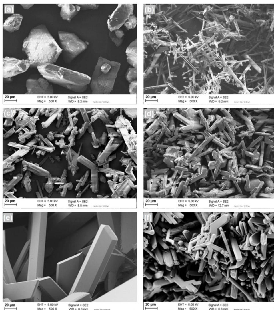
**Figure 7.** SEM images of  $\text{NaHCO}_3$ , comparing commercial crystals (a) with crystals obtained using osmotic membrane distillation crystallization at different temperatures: (b) 15 °C; (c) 20 °C; (d) 30 °C; (e) 35 °C; (f) 40 °C.
