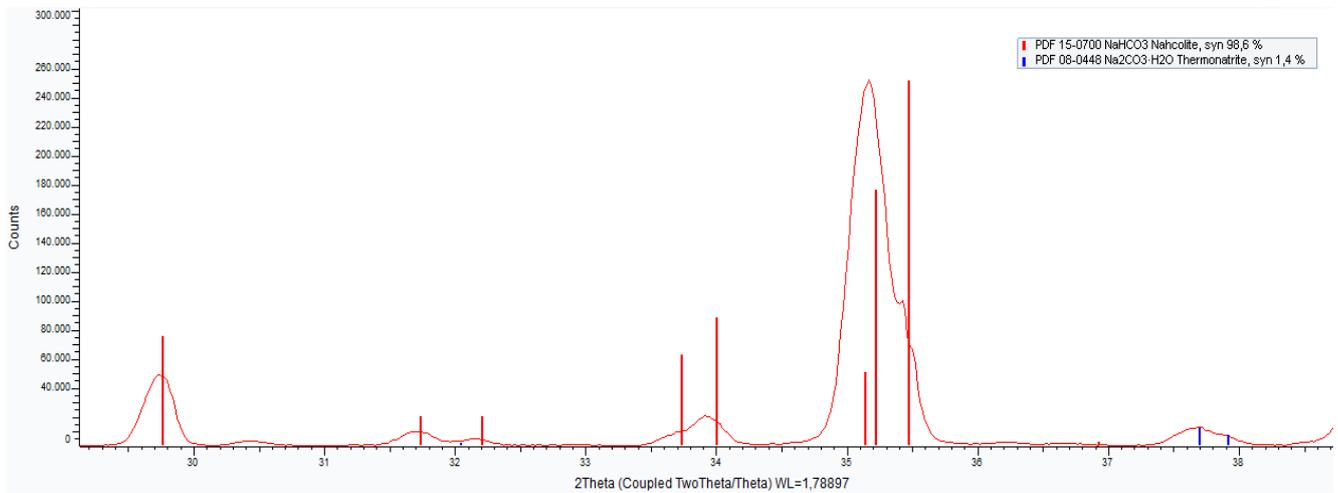
Figure A2. XRD quantitative analysis for crystals produced at 15 °C.
