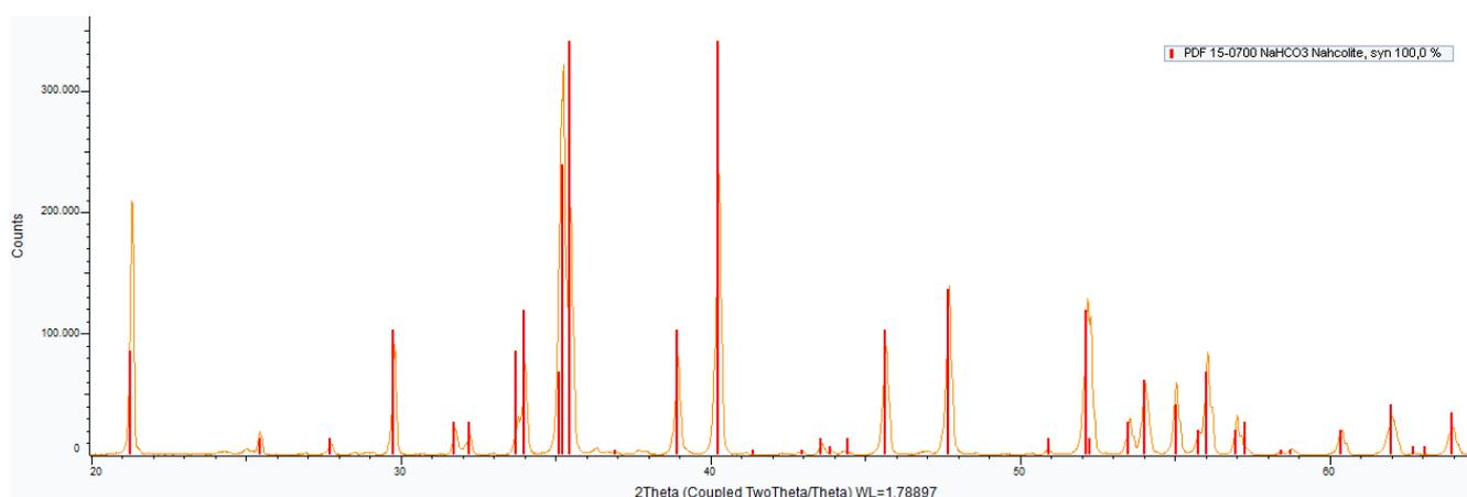
Figure A6. XRD quantitative analysis for crystals produced at 40 °C.
