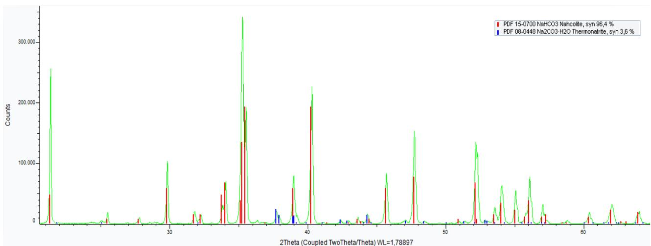
Figure A4. XRD quantitative analysis for crystals produced at 30 °C.
