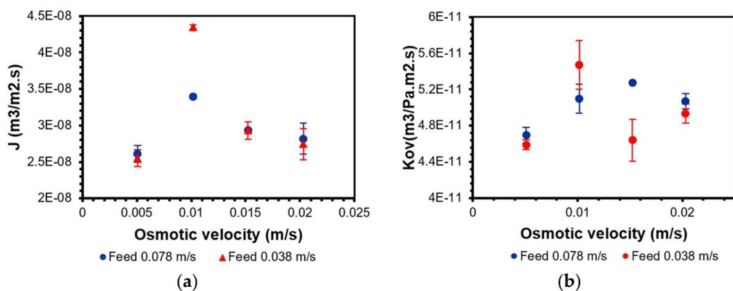
**Figure 4.** (a) Flux for changes in osmotic flow rate. (b)  $K_{ov}$  for changes in osmotic flow rate. The concentration of  $\text{NaHCO}_3$  was at a maximum, and the feed and osmotic solutions were at room temperature.
