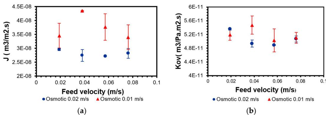
**Figure 3.** Effect of feed and osmotic velocities on (a) flux and (b)  $K_{ov}$ . The concentration of the  $\text{NaHCO}_3$  was at a maximum, and feed and osmotic solutions were at room temperature.
