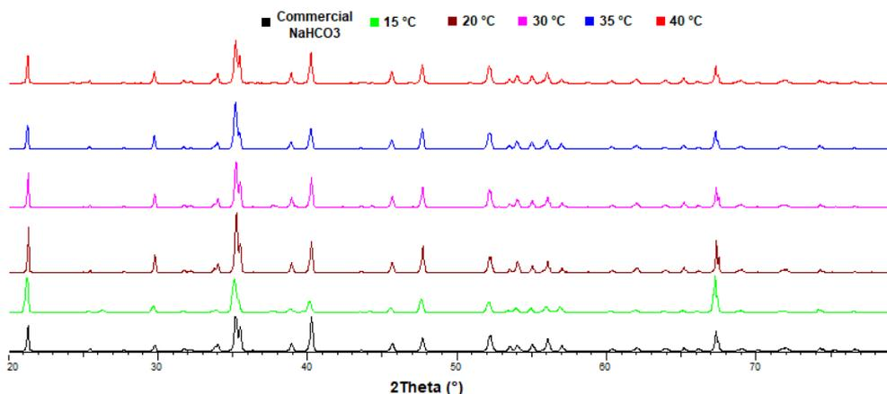
**Figure 8.** NaHCO<sub>3</sub> crystals—X-ray diffraction analysis.
