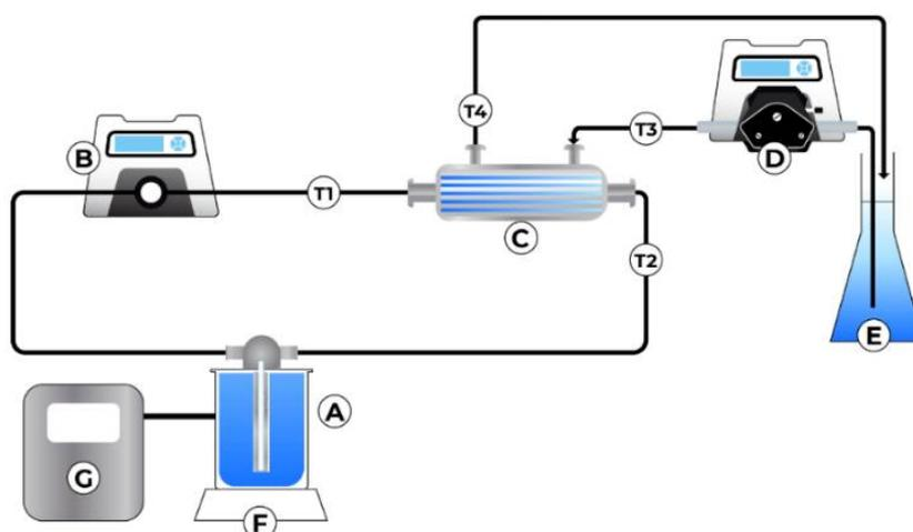
**Figure 2.** Schematic diagram of the membrane distillation crystallization setup: A feed solution; B gear pump; C membrane contactor; D peristaltic pump; E osmotic solution; F balance; G water bath/cooler; T1–T4 thermometers.
