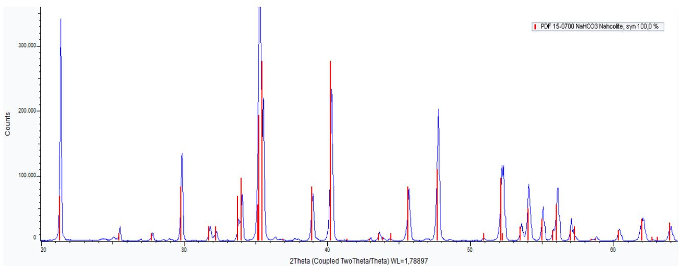
Figure A3. XRD quantitative analysis for crystals produced at 20 °C.
