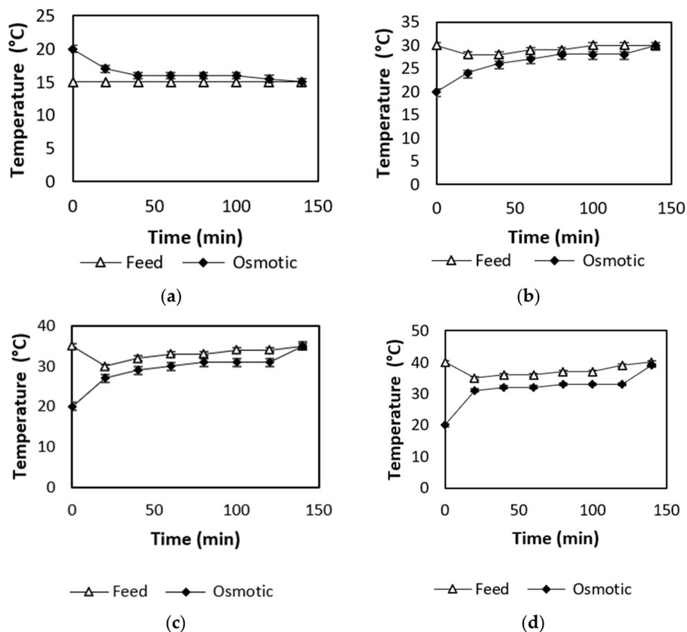
**Figure A1.** Feed and osmotic temperature evolution with time during the thermal evaluation of membrane distillation crystallization: (a) 15 °C; (b) 20 °C; (c) 35 °C; (d) 40 °C.
