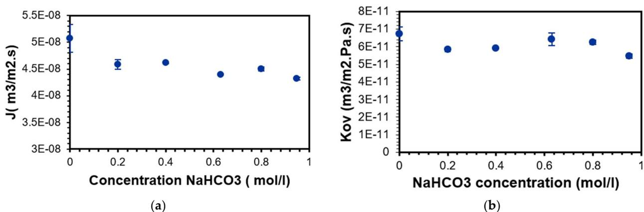
**Figure 5.** Effect of the concentration of  $\text{NaHCO}_3$  in the feed solution on: (a) flux and (b)  $K_{\text{ov}}$ . Feed velocity was 0.038 m/s, osmotic velocity was 0.01 m/s, and osmotic and feed solutions were at room temperature.
