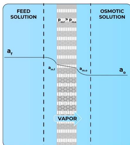
Figure 1. Concentration profiles in osmotic membrane distillation crystallization.
