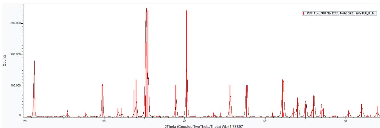
Figure A5. XRD quantitative analysis for crystals produced at 35 °C.
