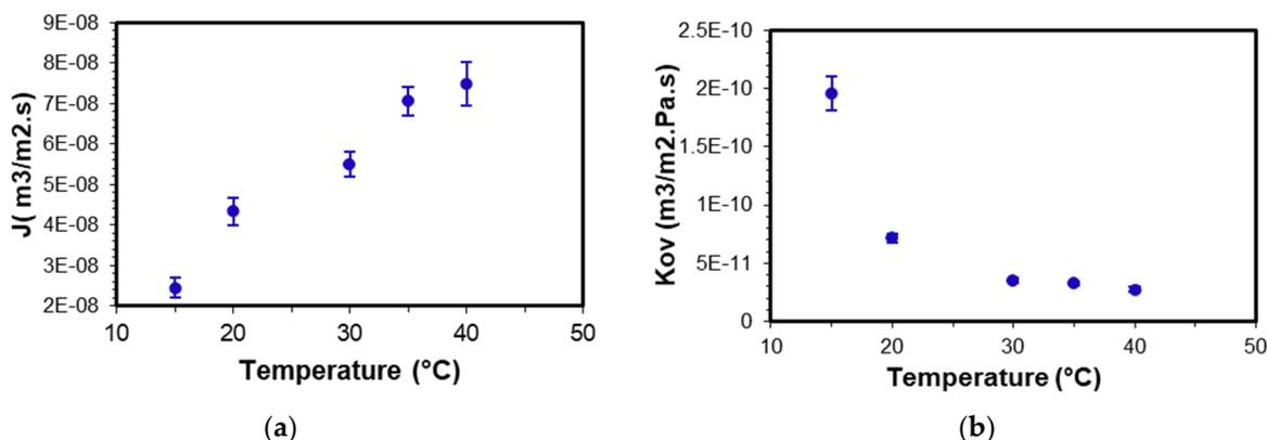
**Figure 6.** (a) Flux for changes in temperature, for 0,8 mol/L of NaHCO<sub>3</sub>. (b) K<sub>ov</sub> for changes in temperature, for 0,8 mol/L of NaHCO<sub>3</sub>.
