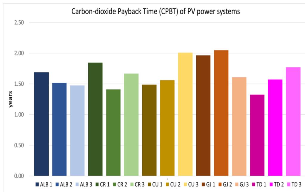
**Figure 7.** Carbon-dioxide Payback Time for the different PV power centers in Castilla—La Mancha.
