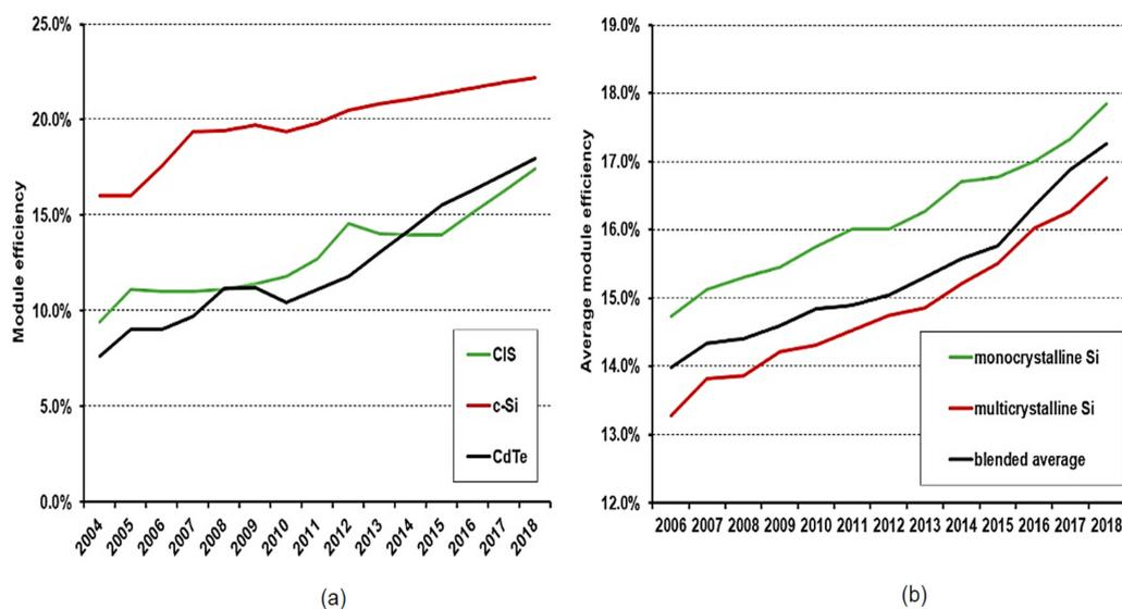
**Figure 2.** (a) Development in efficiency for the top products on the market. (b) Development of average efficiency in crystalline silicon modules [16].
