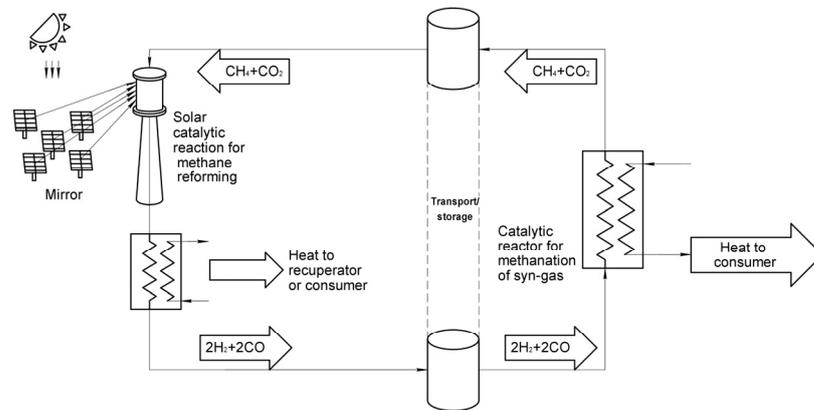
**Figure 16.** Thermochemical accumulation in a solar power plant.
