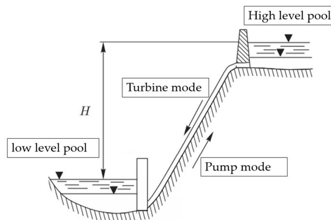
**Figure 5.** Pumped hydroelectric energy storage.
