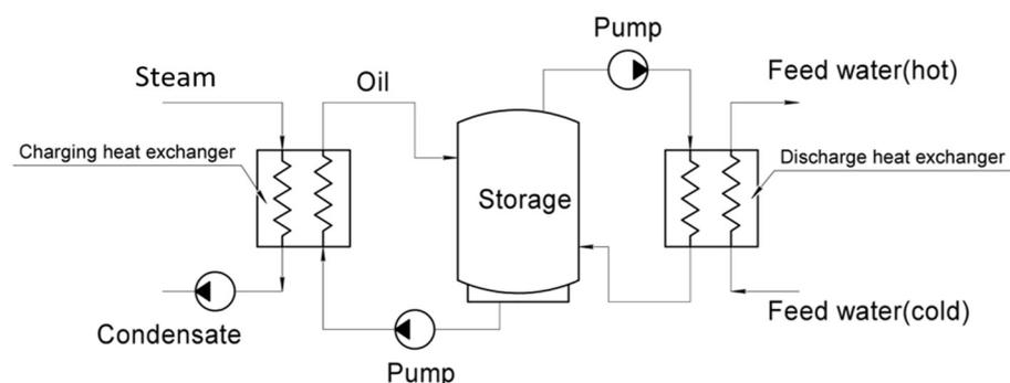
**Figure 13.** Heat flow chart with an intermediate heat carrier.
