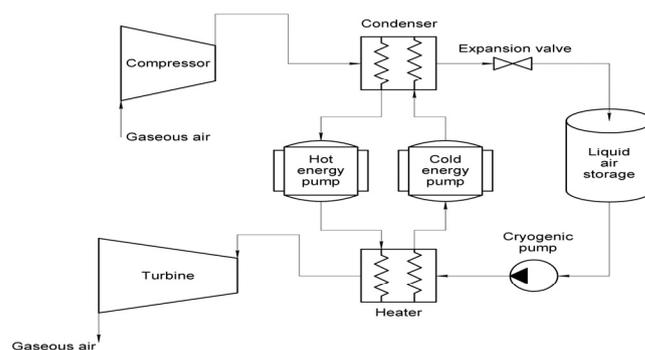
**Figure 21.** Energy accumulation with air liquation.
