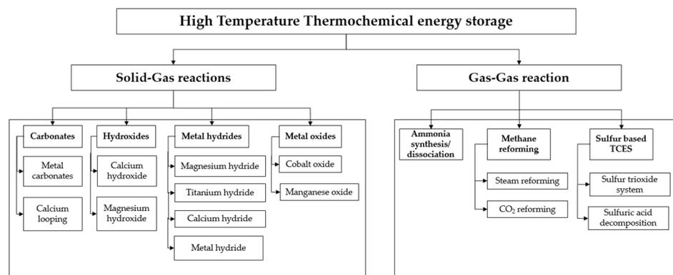
**Figure 8.** Thermochemical accumulation reactions.
