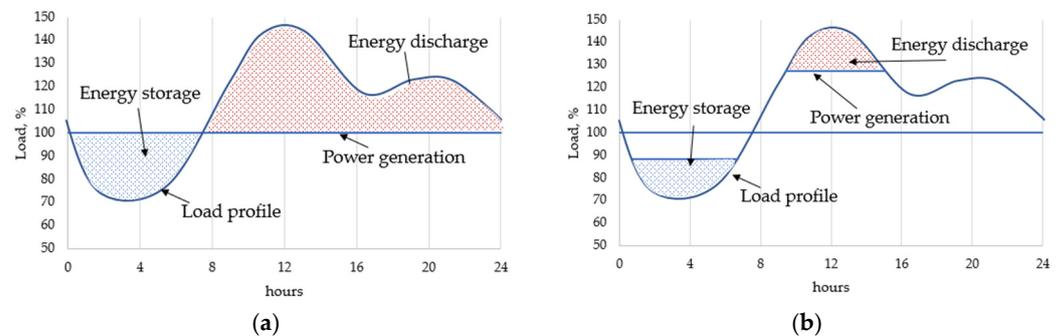
**Figure 1.** Accumulation system operation in a power grid: (a) load leveling; (b) peak shaving.
