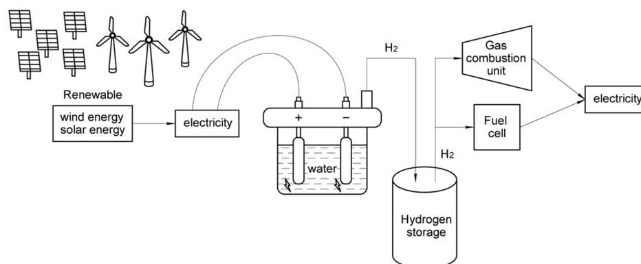
**Figure 7.** Hydrogen energy accumulation scheme.
