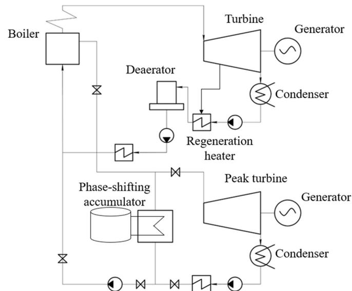
**Figure 14.** Heat flow chart of a TPP with phase transformation accumulator.
