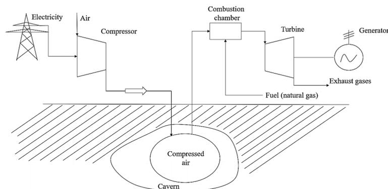
**Figure 6.** Compressed air energy storage system.
