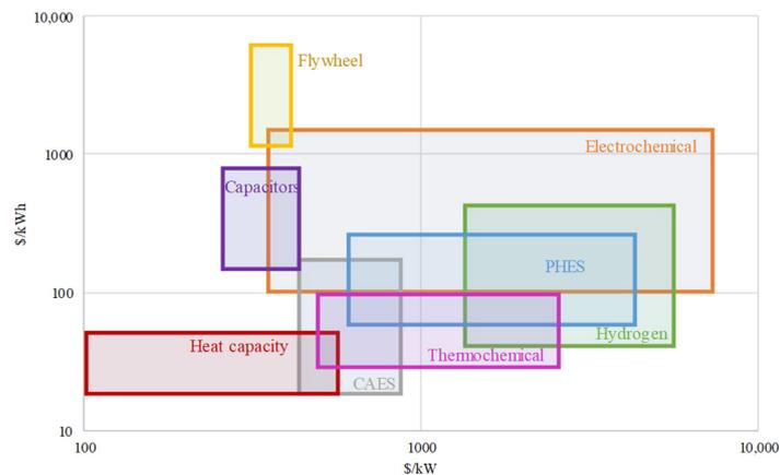
**Figure 10.** Cost of energy accumulation systems.
