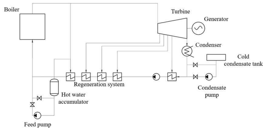
**Figure 11.** Heat flow chart of TPP with feed water accumulator.
