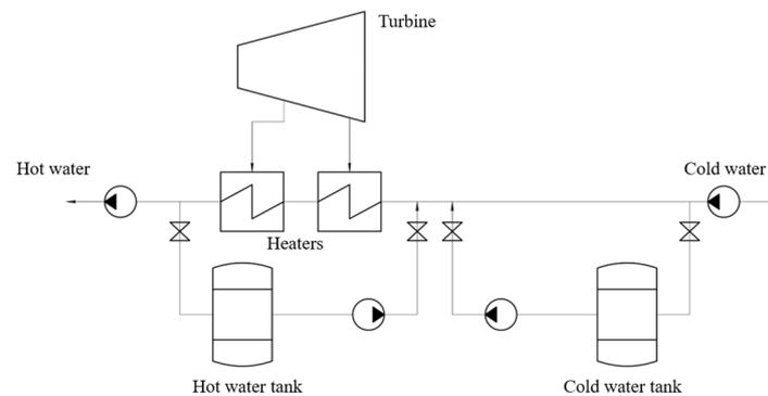
**Figure 12.** Heat flow chart of TPP with heating water accumulator.
