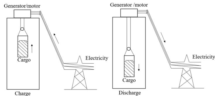
**Figure 4.** Gravitational energy storage system.
