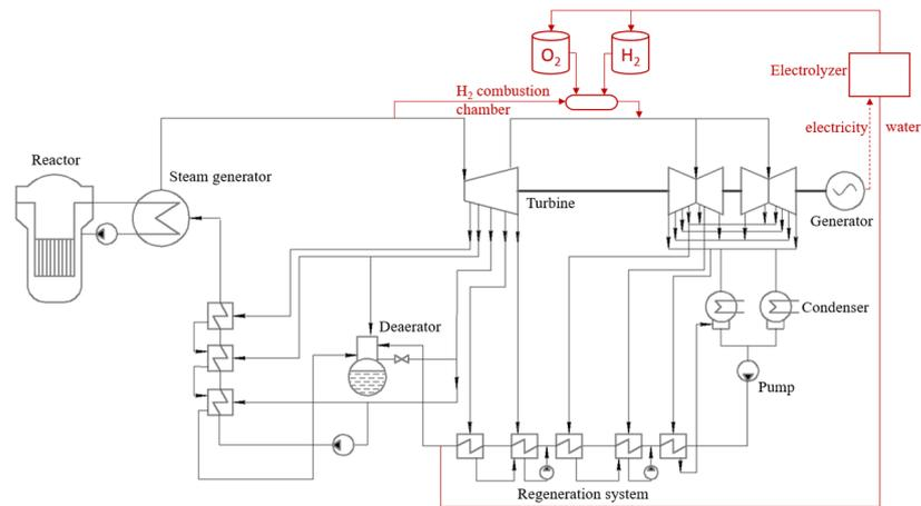
**Figure 18.** Power plant facility equipped with hydrogen accumulation.
