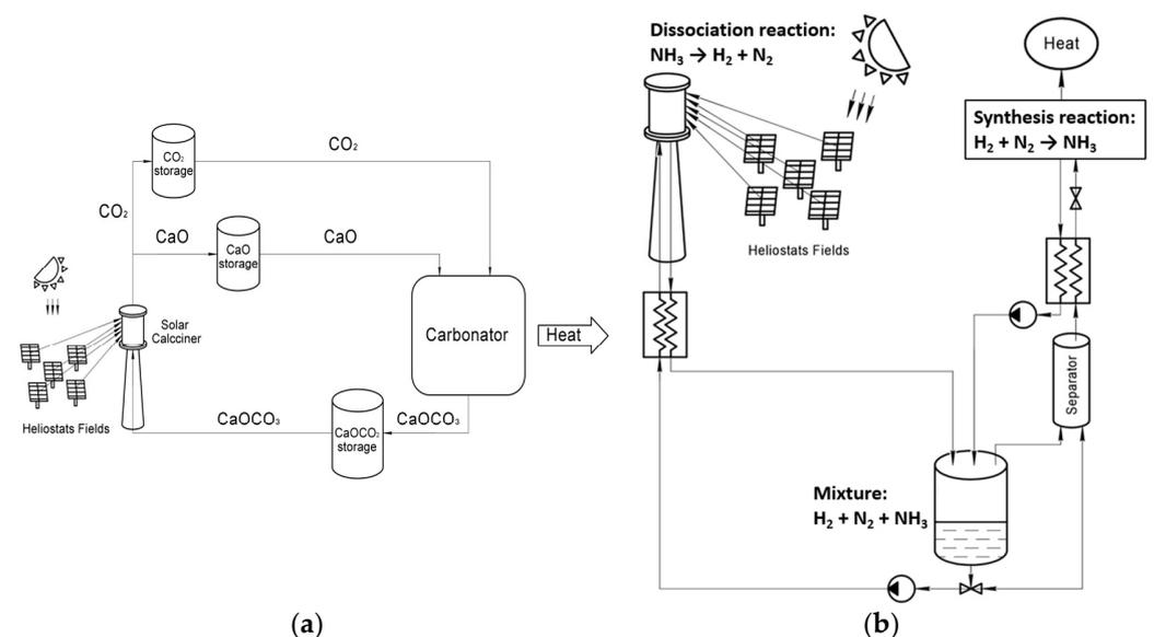
**Figure 15.** Thermochemical accumulation in a solar power plant: (a) calcium carbonate synthesis cycle; (b) ammonia synthesis cycle.
