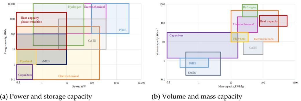
**Figure 9.** Main performance of energy accumulation systems.
