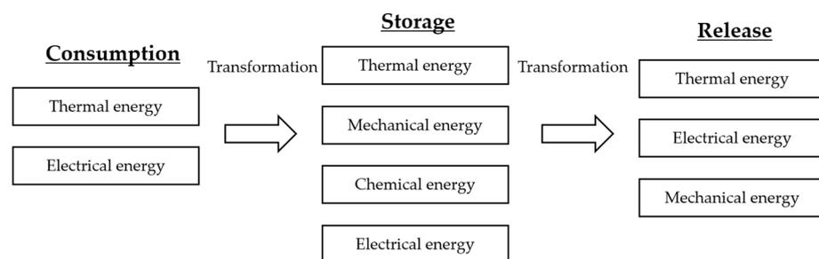
**Figure 2.** Energy transformation sequence of an accumulation system.
