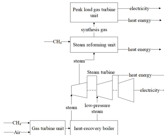
**Figure 17.** Combined cycle facility equipped with methane steam conversion.
