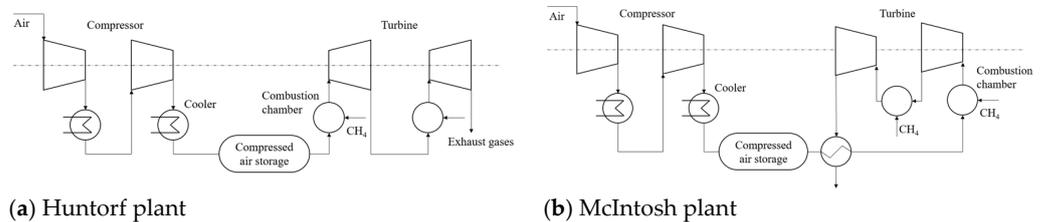
**Figure 19.** Compressed air energy storage systems: (a) Huntorf plant, Germany; (b) McIntosh plant, Alabama, USA.
