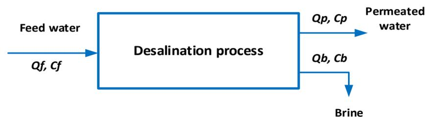
**Figure 5.** Desalination process diagram (author’s elaboration).
