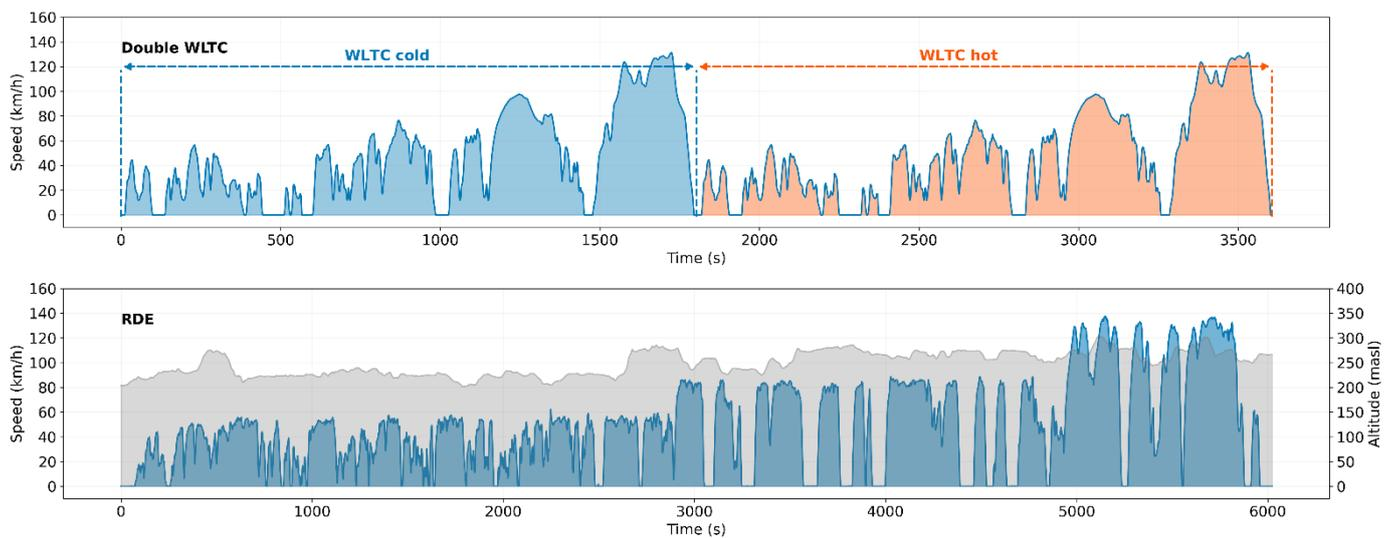
**Figure 1.** Speed profile of the double WLTC tests (**top panel**) and the on-road tests (**bottom panel**). The bottom panel's shaded grey area indicates the altitude profile during the RDE test.
