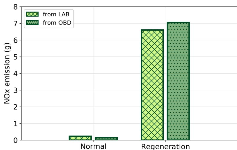
**Figure 7.** The cumulative NOx emissions measured in the laboratory and by OBM in WLTC cycles performed under normal SCR functioning conditions and under DPF regeneration conditions.
