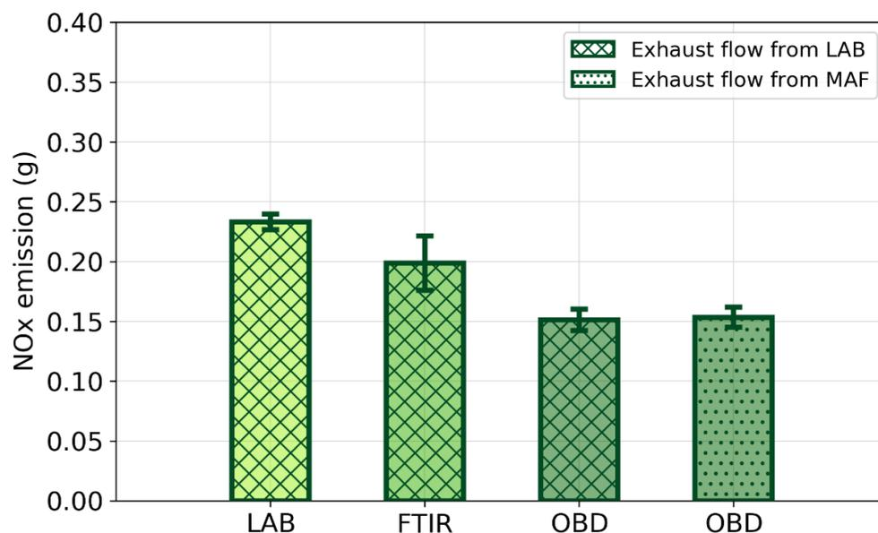
**Figure 5.** Vehicle 1 average of the cumulative NO<sub>x</sub> emissions measured at tailpipe with different methods over two different hot WLTC cycles. LAB, FTIR and OBD indicate that the NO<sub>x</sub> concentration used was measured with standard laboratory equipment, a lab-grade FTIR spectrometer or the on-board NO<sub>x</sub> sensor, respectively. The two different pattern fills indicate which exhaust flow measurement was used, as indicated in the legend.
