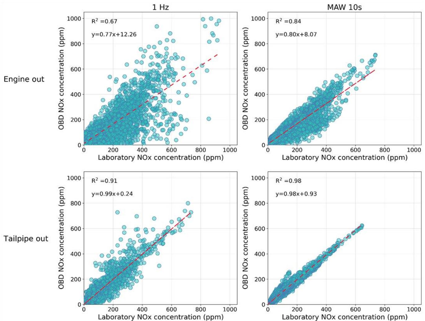
**Figure 4.** Plots showing the correlation between OBD signals and 1 Hz laboratory measurements at the engine-out (top graphs) and tailpipe-out (bottom graphs) of Vehicle 1. Different correlation methods are compared: 1 Hz data in the left-hand-side panels and a 10 s moving average window (MAW) in the right-hand-side panels.
