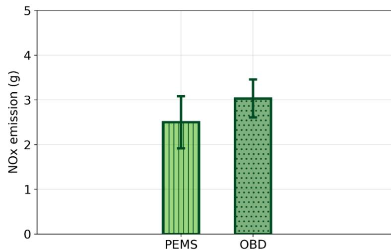
**Figure 6.** Vehicle 2 average of the cumulative NOx emissions measured at tailpipe with a portable emission measurement system (PEMS) and with the on-board NOx sensor (OBD) in 2 RDE-compliant tests.
