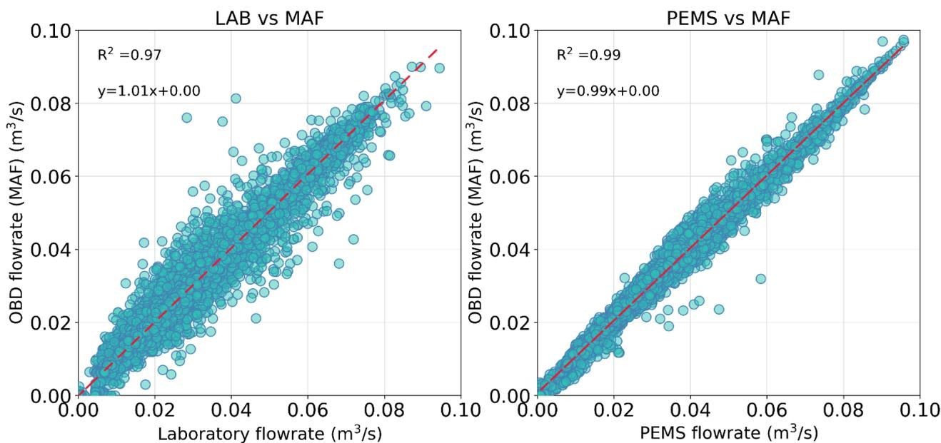
**Figure 2.** (Left panel) Correlation between MAF signal from OBD and flow rate measured in the laboratory (difference between CVS and dilution flow rate) from all the WLTC tests performed. (Right panel) Correlation between MAF and PEMS flow rate from all the on-road tests performed.
