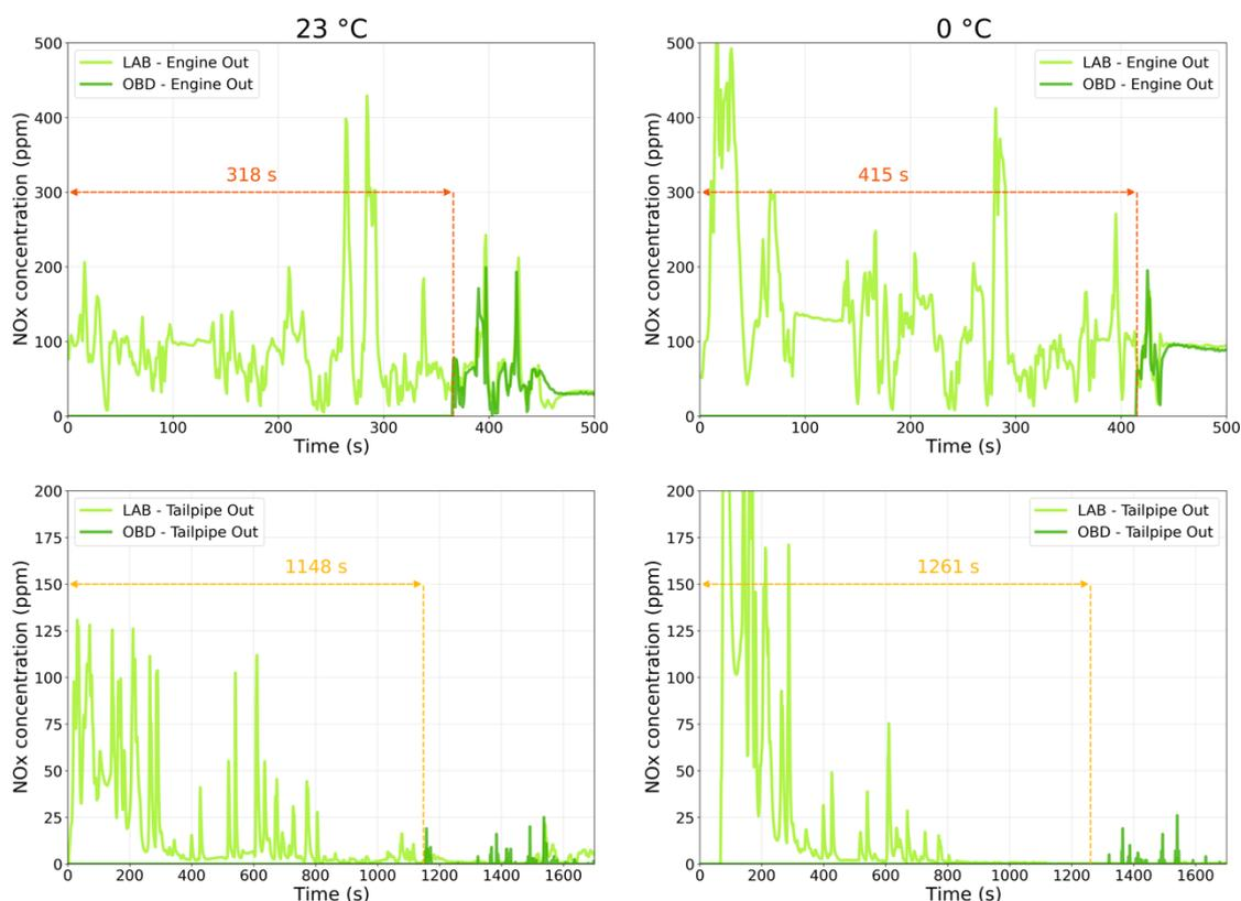
**Figure 3.** Top panels: engine-out NOx concentration signals from the OBD port and as measured in the laboratory (LAB) at 23 °C and 0 °C. Bottom panels: tailpipe-out NOx concentration signals from the OBD port and as measured in the laboratory (LAB) at 23 °C and 0 °C.
