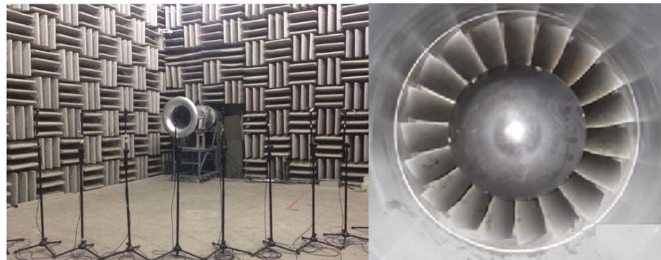
**Figure 3.** Inlet noise measuring section in semi-anechoic chamber and photo of axial flow fan.
