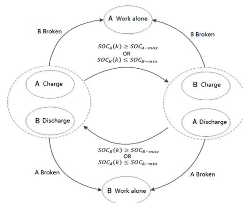
**Figure 4.** Dual-energy storage charge-discharge cooperative working mode.
