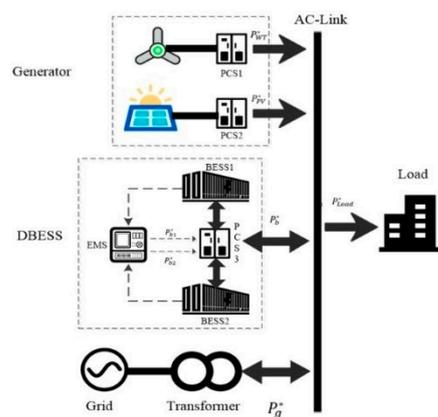
Figure 2. Microgrid architecture with a dual battery energy storage system mode.
