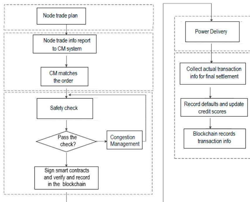
**Figure 5.** Flowchart of the control algorithm proposed for energy blockchain where CM indicates the central matching server.
