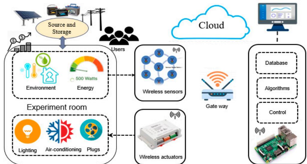
Figure 2. Building monitoring and control system architecture.
