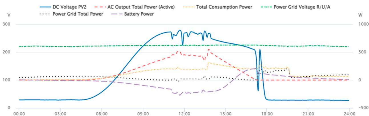
Figure 16. Power flows through inverter in 4 November 2021.
